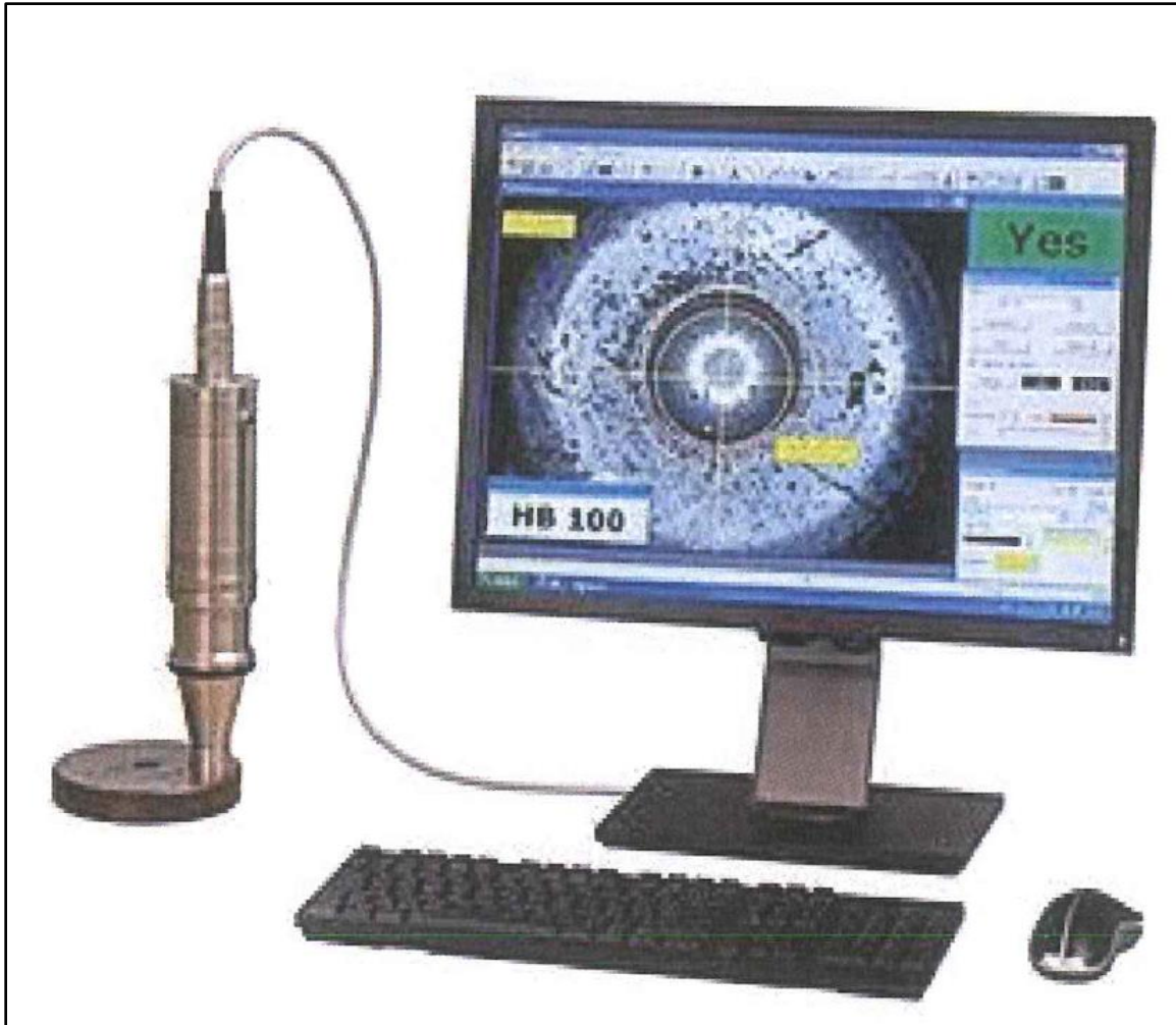
Figure 4.7 Image of On-site Hardness HB100 Digital Microscope. Provided by ApplusRTD Norway.
