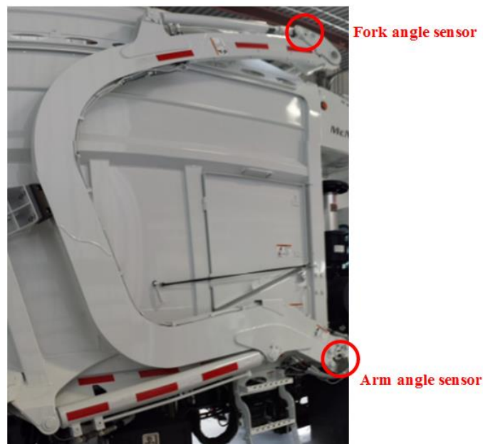
Figure 13: The test system is shown with both the arm and fork cylinders fully retracted and the two
