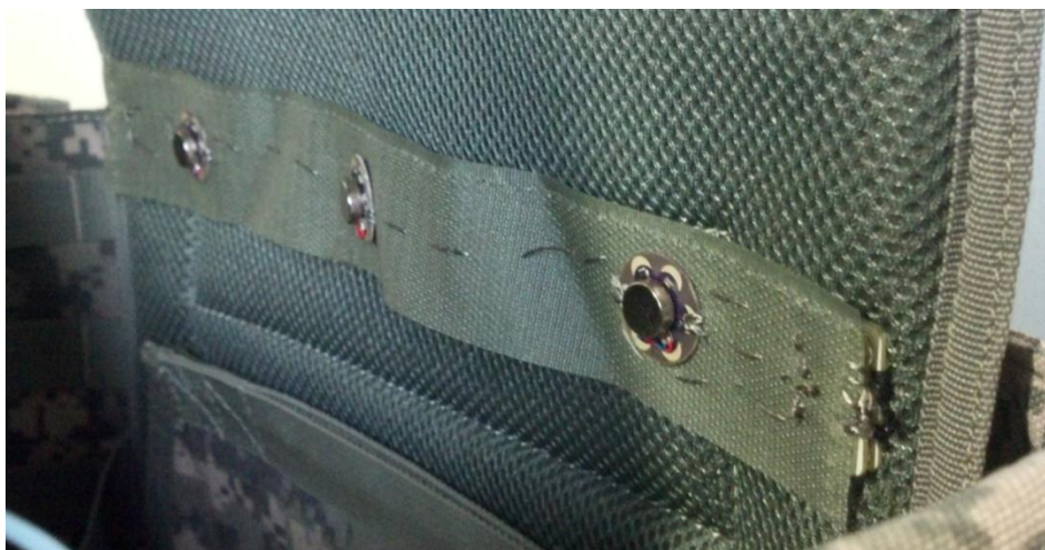
Figure 11: Vibrotactile motors mounted in the T3V
