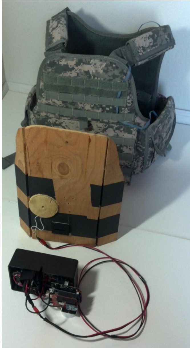
Figure 14: The T3V with the tactor mounted on the insert, and the required circuitry and microcontroller contained within the enclosure
