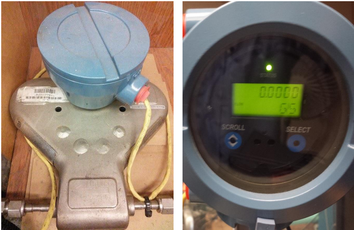
Figure 3.9 Fuel Flow Meter and Display Unit
