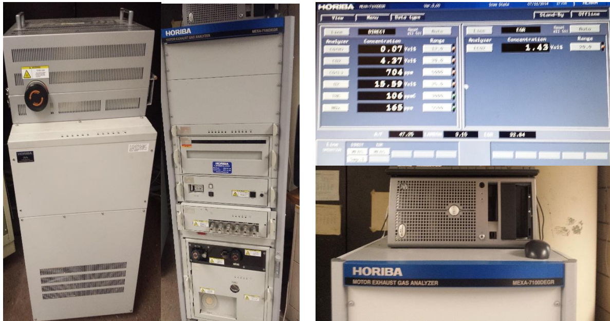
Figure 3.1 Horiba MEXA7100 DEGR Exhaust Gas Analyzer
