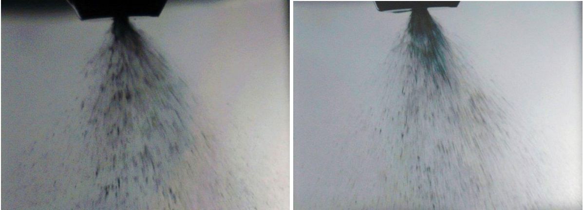
Figure 8: Canola oil spray with atomizing air at 25 psi (left) and 35 psi (right).
