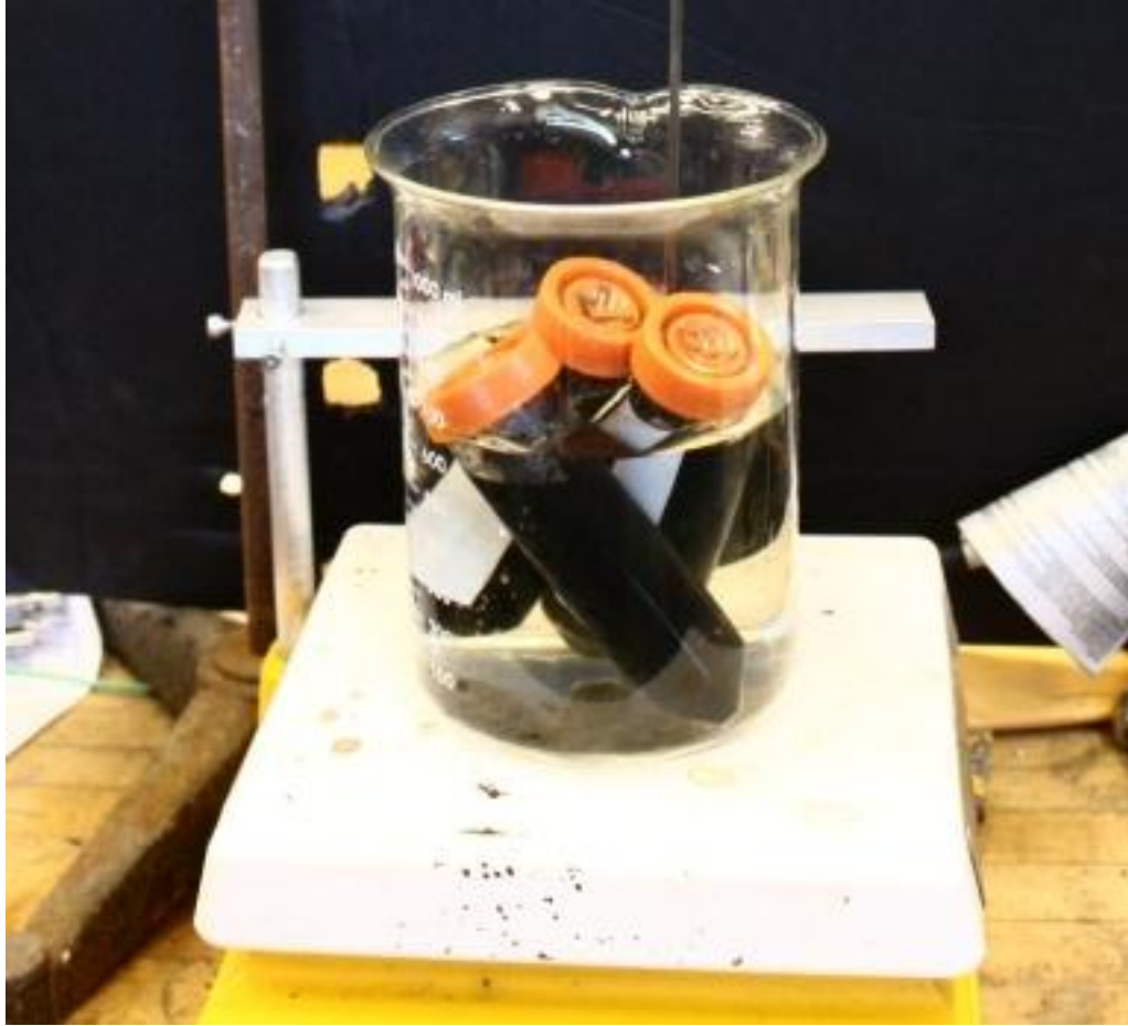
Figure 3 Pyrolysis oil mixed with ethanol in aging setup.
