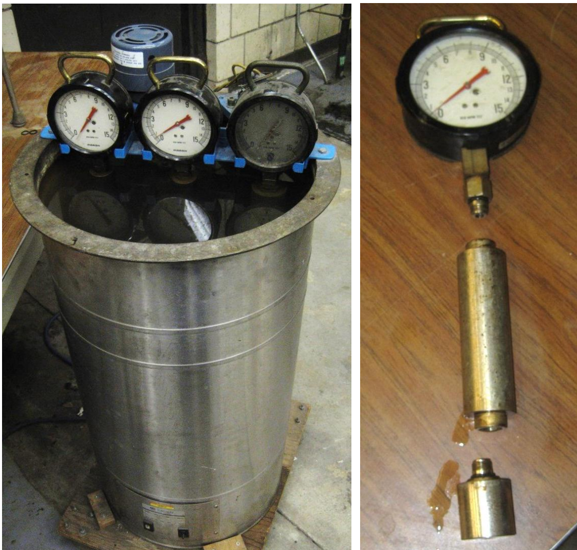
Figure 23: Reid vapor pressure test apparatus, including water bath (left) and chamber (right).
