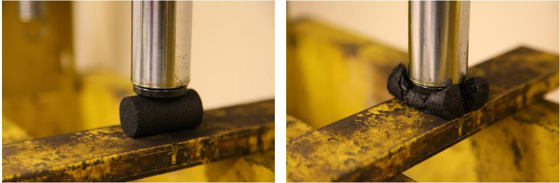
Figure 17: Indirect tensile strength test before (left) and after (right)
