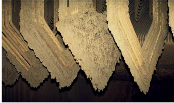
Figure 3: Deposit build-up on superheaters after one week of co-firing coal and straw [17]
