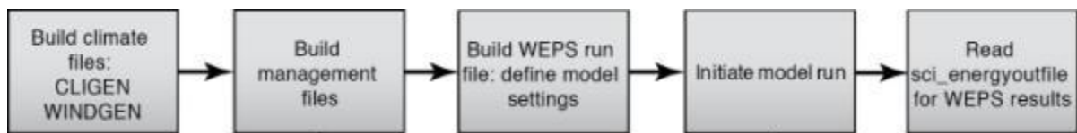
Figure 2.9. The WEPS model wrapper within the toolkit utilizes the data provided through the previously described models to perform all necessary functions setting up the WEPS model run scenario.
