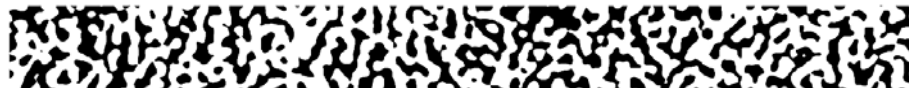
Figure 3.1: Morphology of the active layer for a typical donor-acceptor system imaged using TEM [6]. Dimensions are 1200nm \times 100nm.
