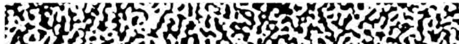
Figure 2.1: Cross-sectional morphology for rrP3HT:PCBM system imaged using TEM[6]. Dimensions are 1200\text{nm} \times 100\text{nm} . The white regions represent the photo active polymer (rrP3HT), while the black regions represent the conducting fullerene (PCBM).
