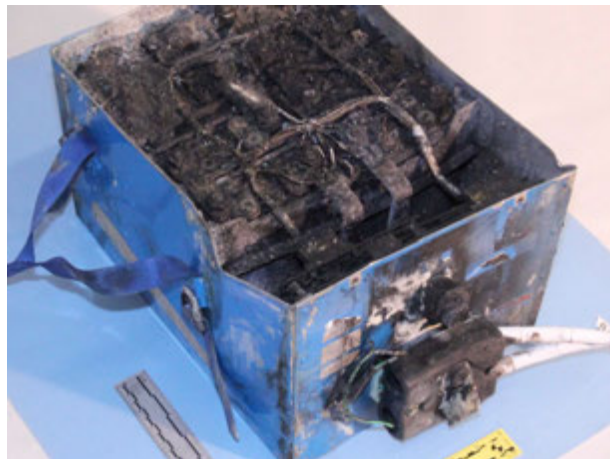
Figure 1.2 Burned Li-ion Polymer battery from Boeing 787 Dreamliner
