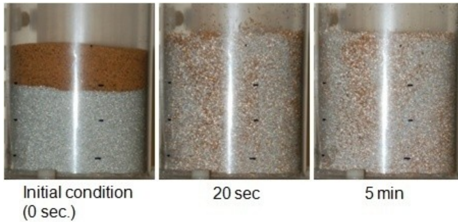
Figure E. 20: Photographs of experiments with 25% 500-600 \mu\text{m} GWS mixed with 75% 500-600 \mu\text{m} GB and fluidized at U_g = 2 U_{mf} with dry air in the 9.5 cm ID FBR at the specified intervals.
