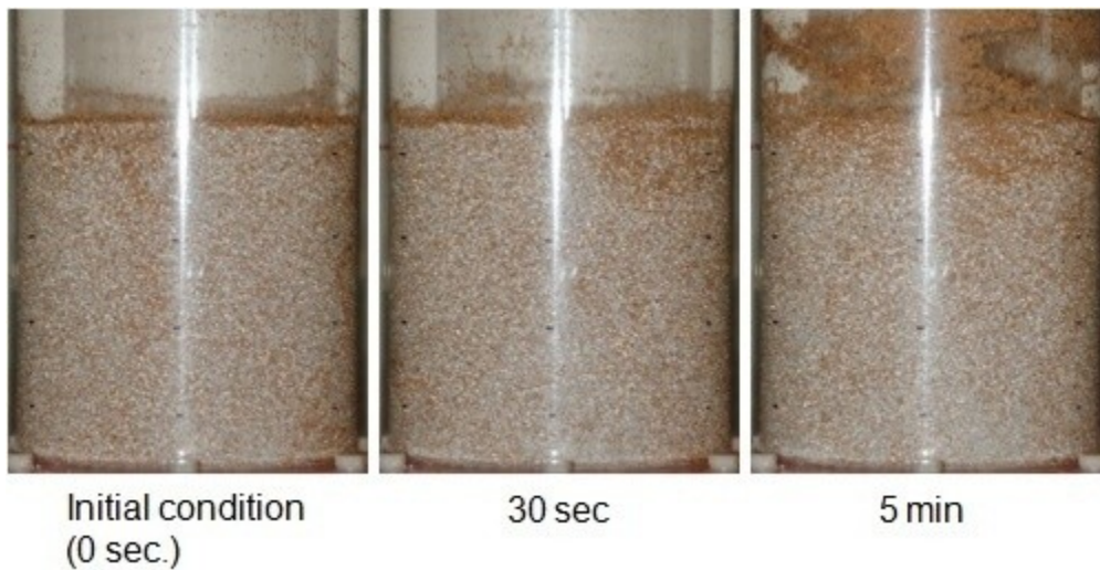
Figure E. 38: Photographs of experiments with 25% 500-600 \mu\text{m} GWS mixed with 75% 500-600 \mu\text{m} GB and fluidized at U_g = 1.5 U_{mf} with dry air in the 15.2 cm ID FBR at the specified intervals.
