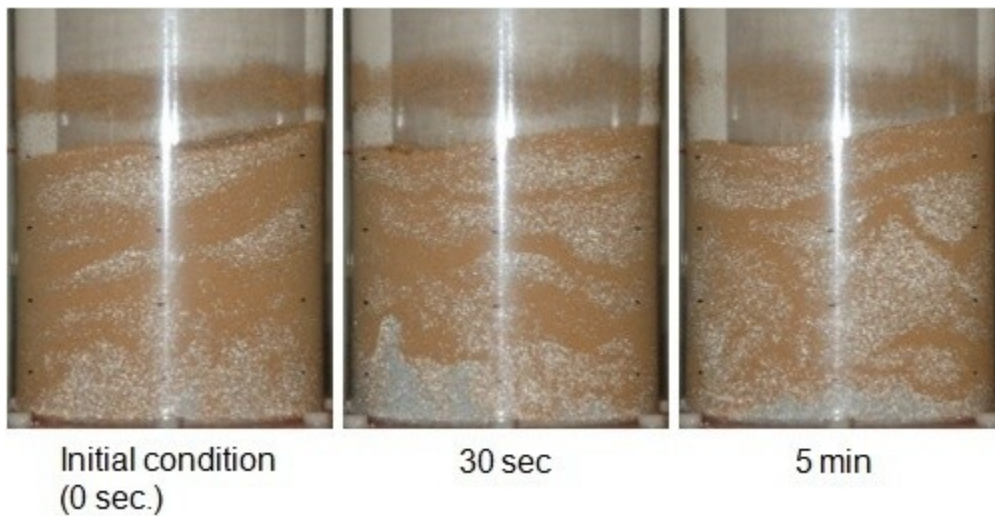
Figure E. 34: Photographs of experiments with 25% 212-300 μm GWS mixed with 75% 500-600 μm GB and fluidized at U_g = 1.2 U_{mf} with dry air in the 15.2 cm ID FBR at the specified intervals.
