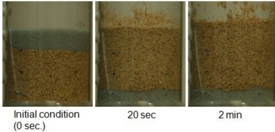
Figure E. 13: Photographs of experiments with 75% 500-600 \mu\text{m} GCC mixed with 25% 500-600 \mu\text{m} GB and fluidized at U_g = 2 U_{mf} with humidified air in the 9.5 cm ID FBR at the specified intervals.
