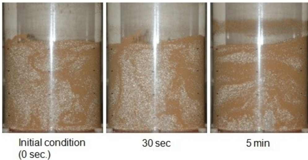
Figure E. 32: Photographs of experiments with 25% 212-300 \mu\text{m} GWS mixed with 75% 500-600 \mu\text{m} GB and fluidized at U_g = 1.5 U_{mf} with humidified air in the 15.2 cm ID FBR at the specified intervals.
