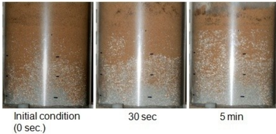
Figure E. 16: Photographs of experiments with 25% 212-300 \mu\text{m} GWS mixed with 75% 500-600 \mu\text{m} GB and fluidized at U_g = 2 U_{mf} with humidified air in the 9.5 cm ID FBR at the specified intervals.
