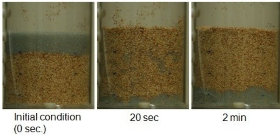
Figure E. 14: Photographs of experiments with 75% 800-1000 \mu\text{m} GCC mixed with 25% 500-600 \mu\text{m} GB and fluidized at U_g = 2 U_{mf} with humidified air in the 9.5 cm ID FBR at the specified intervals.
