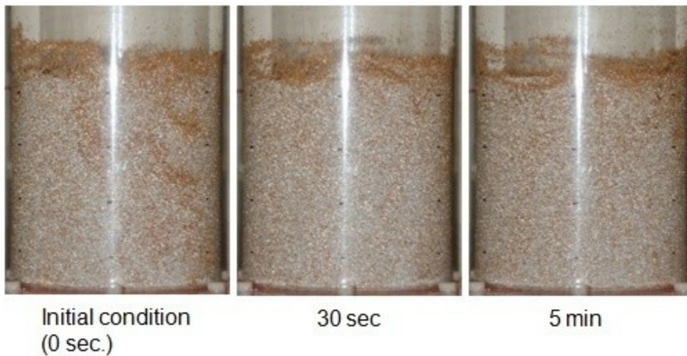
Figure E. 36: Photographs of experiments with 25% 500-600 \mu\text{m} GWS mixed with 75% 500-600 \mu\text{m} GB and fluidized at U_g = 2 U_{mf} with humidified air in the 15.2 cm ID FBR at the specified intervals.
