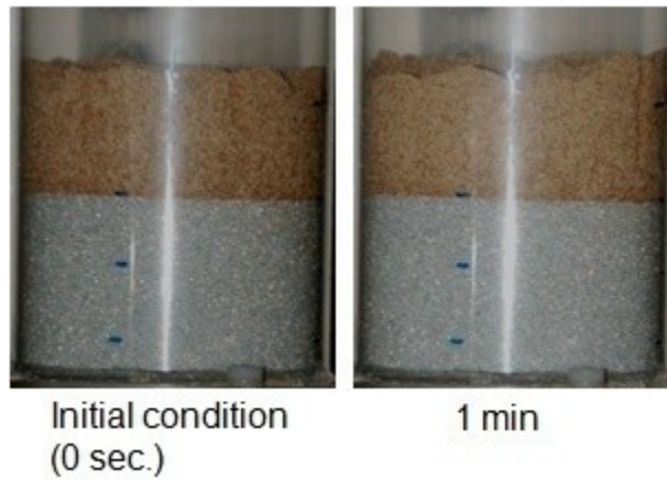
Figure E. 4: Photographs of experiments with 25% 212-300 μm GCC mixed with 75% 500-600 μm GB and fluidized at U_g = 1.5 U_{mf} with humidified air in the 9.5 cm ID FBR at the specified intervals.
