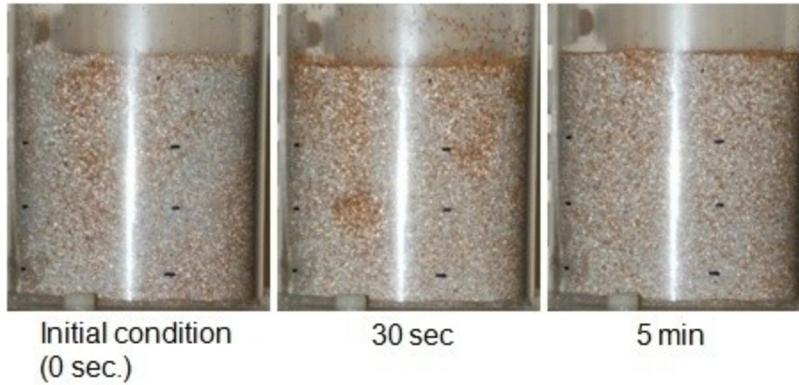
Figure E. 21: Photographs of experiments with 25% 500-600 \mu\text{m} GWS mixed with 75% 500-600 \mu\text{m} GB and fluidized at U_g = 2 U_{mf} with humidified air in the 9.5 cm ID FBR at the specified intervals.
