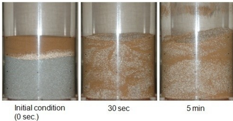
Figure E. 30: Photographs of experiments with 25% 212-300 \mu\text{m} GWS mixed with 75% 500-600 \mu\text{m} GB and fluidized at U_g = 2 U_{mf} with dry air in the 15.2 cm ID FBR at the specified intervals.
