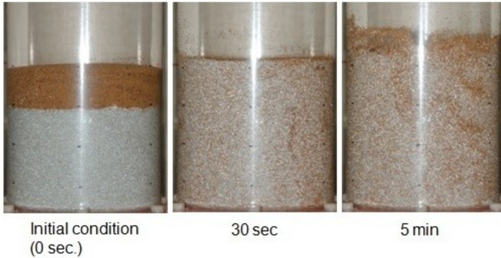
Figure E. 35: Photographs of experiments with 25% 500-600 \mu\text{m} GWS mixed with 75% 500-600 \mu\text{m} GB and fluidized at U_g = 2 U_{mf} with dry air in the 15.2 cm ID FBR at the specified intervals.
