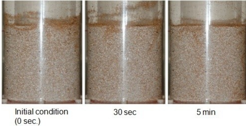
Figure E. 37: Photographs of experiments with 25% 500-600 \mu\text{m} GWS mixed with 75% 500-600 \mu\text{m} GB and fluidized at U_g = 1.5 U_{mf} with humidified air in the 15.2 cm ID FBR at the specified intervals.
