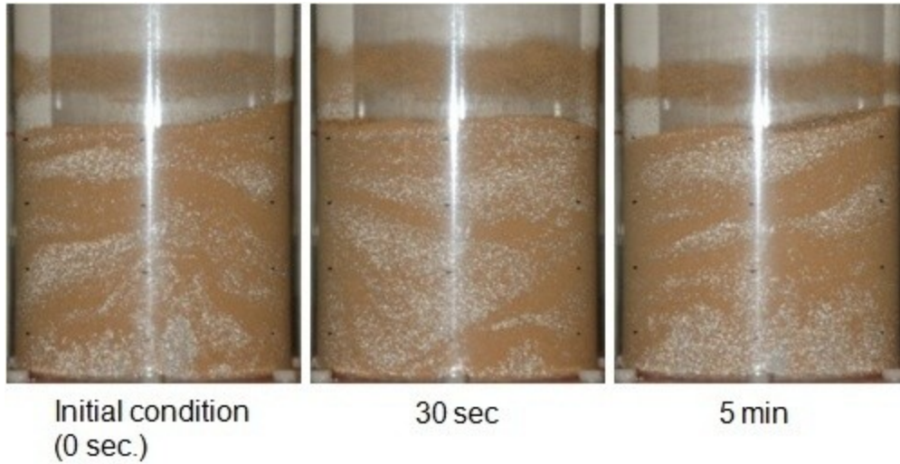
Figure E. 33: Photographs of experiments with 25% 212-300 μm GWS mixed with 75% 500-600 μm GB and fluidized at U_g = 1.5 U_{mf} with dry air in the 15.2 cm ID FBR at the specified intervals.
