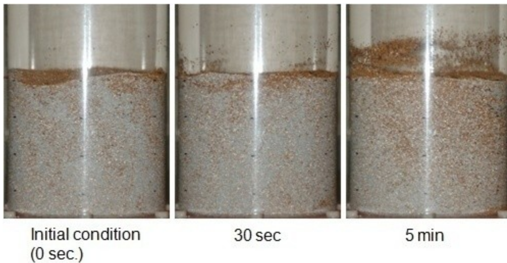
Figure E. 44: Photographs of experiments with 25% 800-1000 \mu\text{m} GWS mixed with 75% 500-600 \mu\text{m} GB and fluidized at U_g = 1.5 U_{mf} with dry air in the 15.2 cm ID FBR at the specified intervals.
