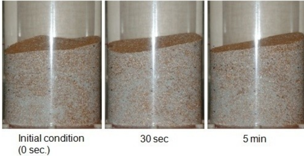
Figure E. 41: Photographs of experiments with 25% 800-1000 \mu\text{m} GWS mixed with 75% 500-600 \mu\text{m} GB and fluidized at U_g = 2 U_{mf} with humidified air in the 15.2 cm ID FBR at the specified intervals.
