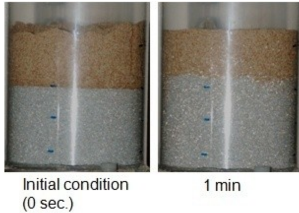
Figure E. 5: Photographs of experiments with 25% 212-300 \mu\text{m} GCC mixed with 75% 500-600 \mu\text{m} GB and fluidized at U_g = 2.6 U_{mf} with humidified air in the 9.5 cm ID FBR at the specified intervals.
