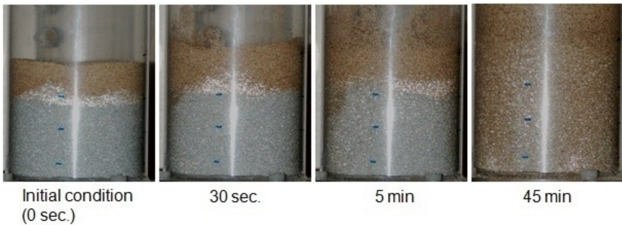
Figure E. 1: Photographs of experiments with 25% 212-300 \mu\text{m} GCC mixed with 75% 500-600 \mu\text{m} GB and fluidized at U_g = 2 U_{mf} with dry air in the 9.5 cm ID FBR at the specified intervals.
