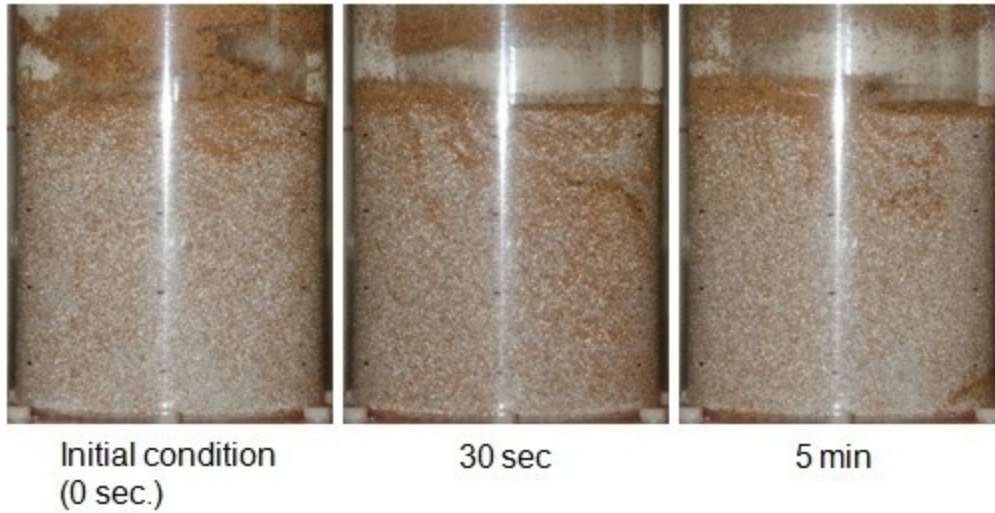
Figure E. 39: Photographs of experiments with 25% 500-600 \mu\text{m} GWS mixed with 75% 500-600 \mu\text{m} GB and fluidized at U_g = 1.2 U_{mf} with dry air in the 15.2 cm ID FBR at the specified intervals.
