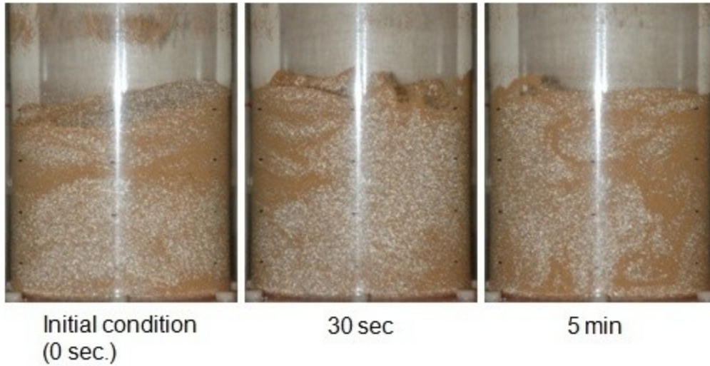
Figure E. 31: Photographs of experiments with 25% 212-300 \mu\text{m} GWS mixed with 75% 500-600 \mu\text{m} GB and fluidized at U_g = 2 U_{mf} with humidified air in the 15.2 cm ID FBR at the specified intervals.
