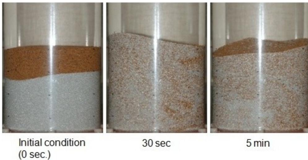
Figure E. 40: Photographs of experiments with 25% 800-1000 \mu\text{m} GWS mixed with 75% 500-600 \mu\text{m} GB and fluidized at U_g = 2 U_{mf} with dry air in the 15.2 cm ID FBR at the specified intervals.
