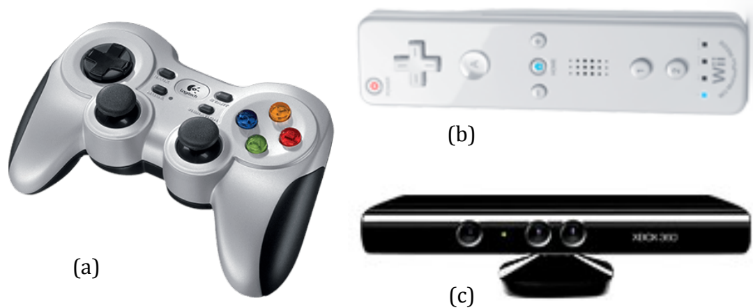
Figure 2. a) The gamepad offers numerous button combinations due to ergonomic design for ease of use and improved learning. ( http://gaming.logitech.com/en-us/product/f710-wireless-gamepad ) b) Wii Remote™ offers one-handed interaction with a series of buttons and positional tracking. ( http://www.nintendo.co.jp/wii/index.html ) c) The Kinect™ offers touch-free interaction through an infrared array of points and two cameras to capture the movements of users to control the interaction. ( http://www.xbox.com/en-US/kinect )
