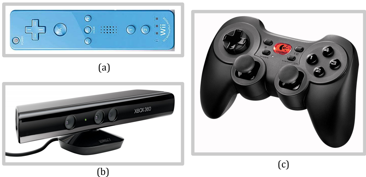
Figure 1. (a) The Nintendo® Wii Remote™ is a COTS device that operates via one-handed navigation. ( www.ic4uae.com/Product.aspx?productid=63005 ) (b) The Microsoft® Kinect™ is a COTS device that operates via touch-free navigation. ( annporter.wordpress.com/2012/04/10/interior-design-via-kinect/ ) (c) The gamepad is a COTS device that operates via two-handed navigation. ( compactiongames.about.com/od/hardware/tp/gamepads.htm )
