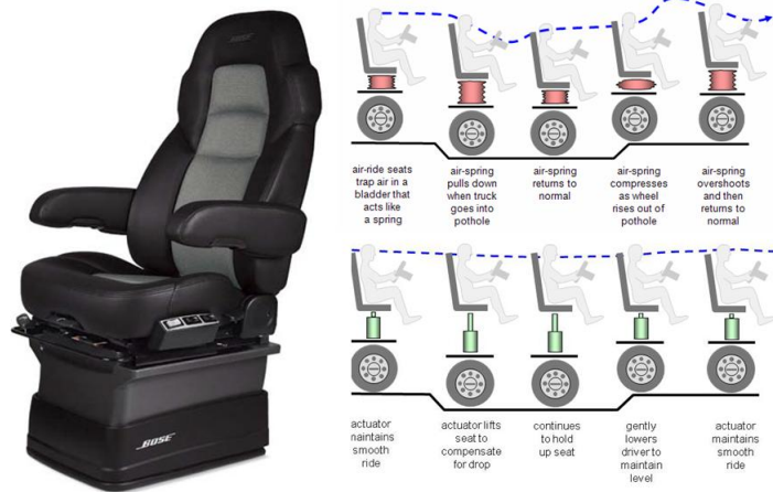
Figure 1.3: Bose Ride System and Its Performance ( http://www.bose.com )
