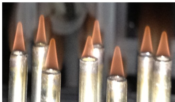
Fig. 4.1. (a) Schematic of eight port tube burner and (b) instantaneous flame image for case E\%NH_3 = 50 at \phi = 1.0 .
