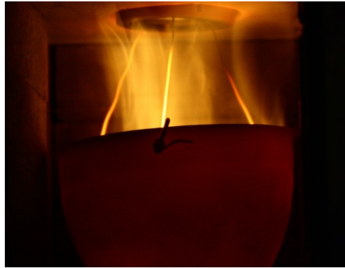
Fig. 2.17. Instantaneous flame image of 100% NH 3 swirl-stabilized turbulent flame. 4
