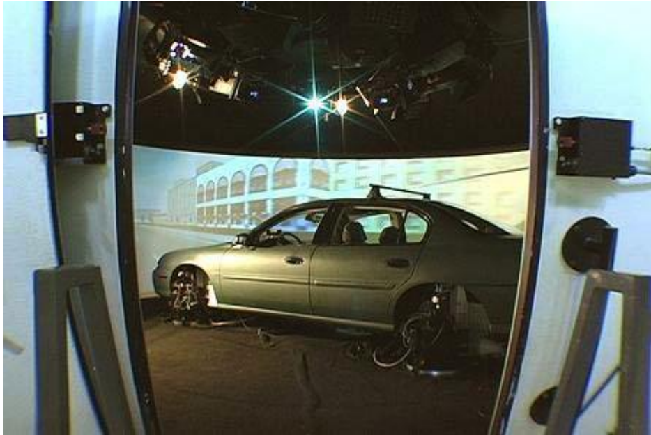
Figure 5: Hydraulic Actuators and Car Cab Inside NADS-1 Dome
