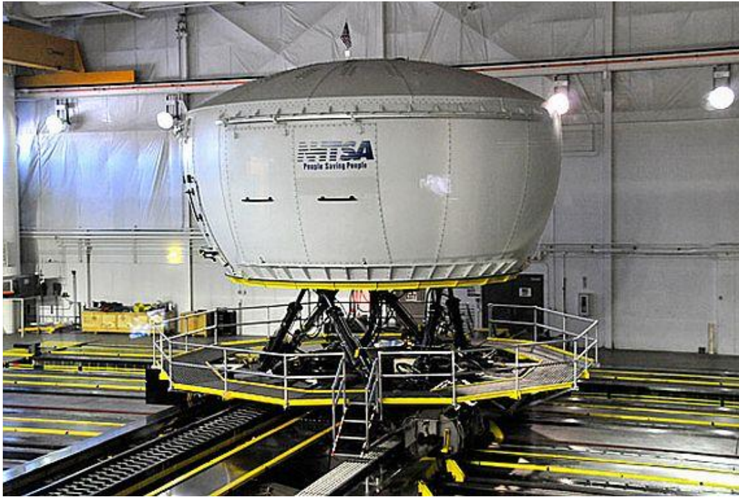
Figure 3: NADS-1 Motion Base
