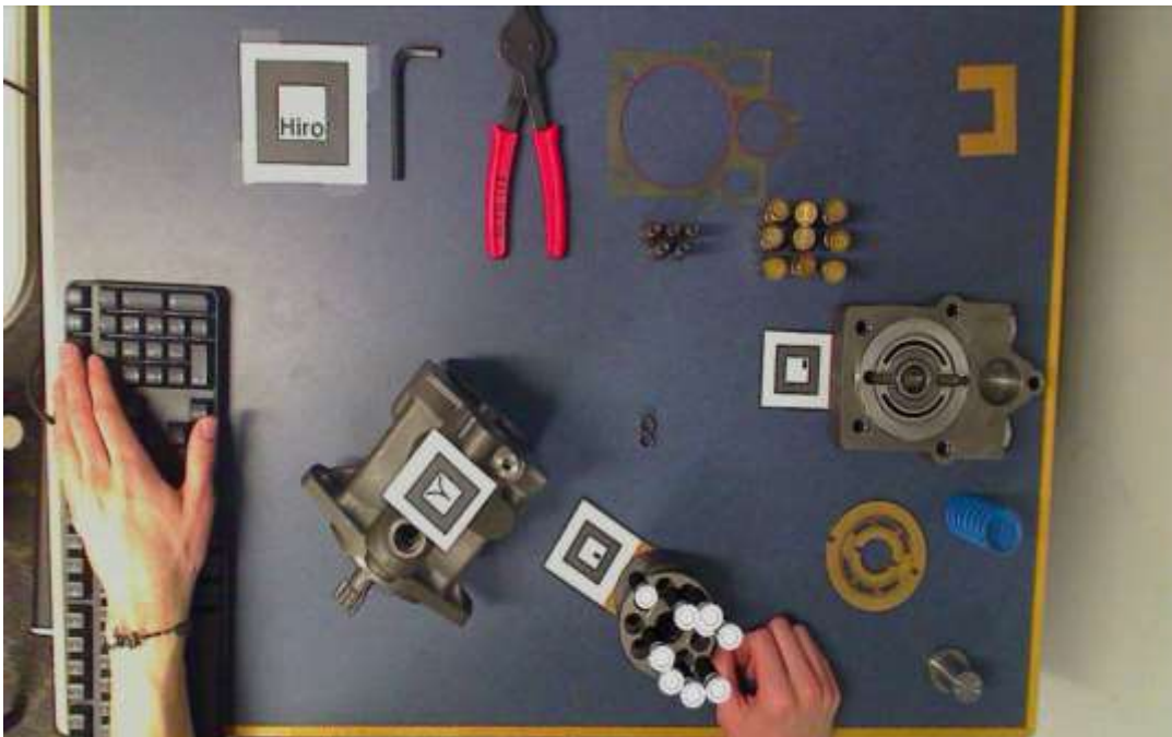
Step 8 – Pistons animate into cylinder block, opposing sides first.
