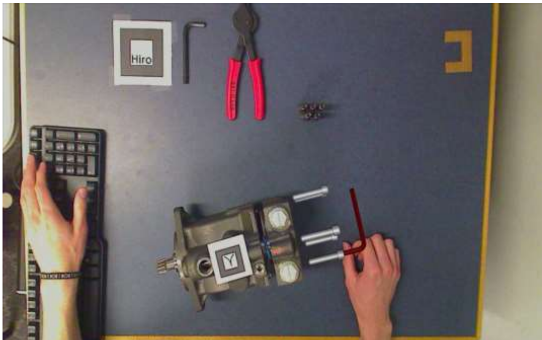
Step 16 – Screws animate into end cap and housing with occlusion. Hex key rotates.
