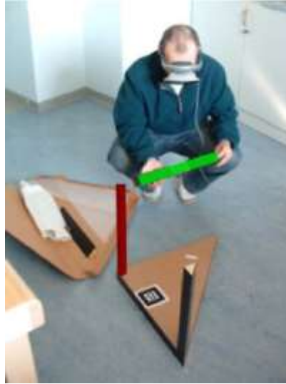
Figure 13. Example of using a 3D model to indicate part manipulation [24].
