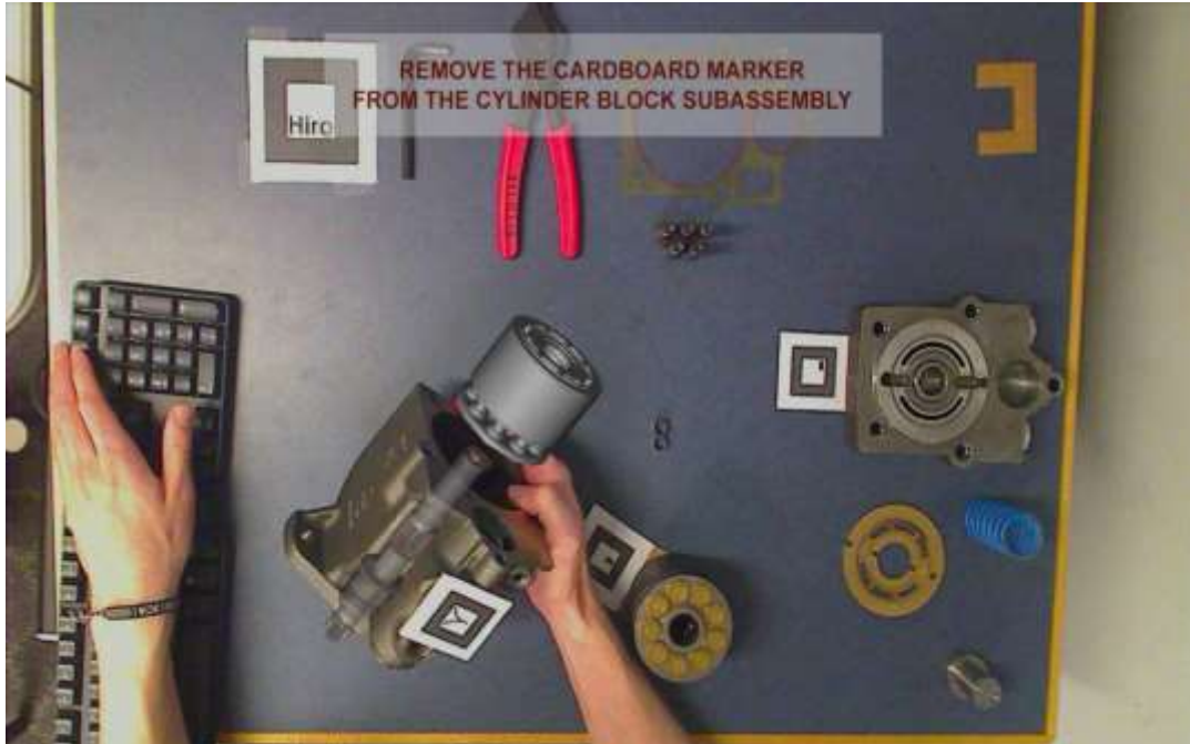
Step 9 – Cylinder block animates onto shaft without occlusion. (Text instructions are not considered an actual assembly step.)
