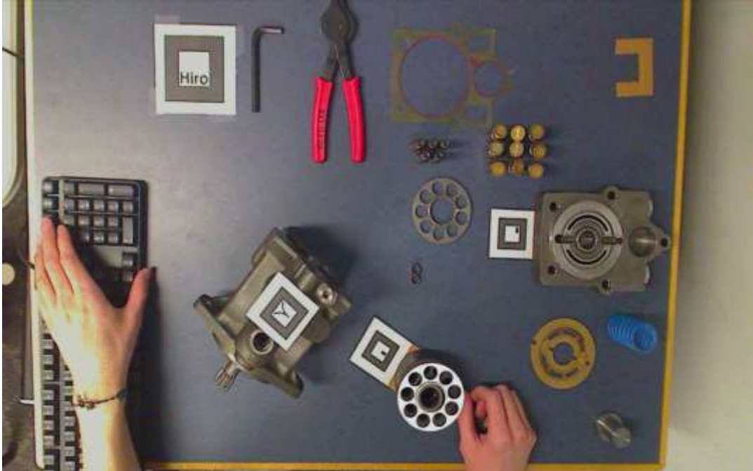
Step 7 – Retainer animates onto retainer guide and rotates to align holes.
