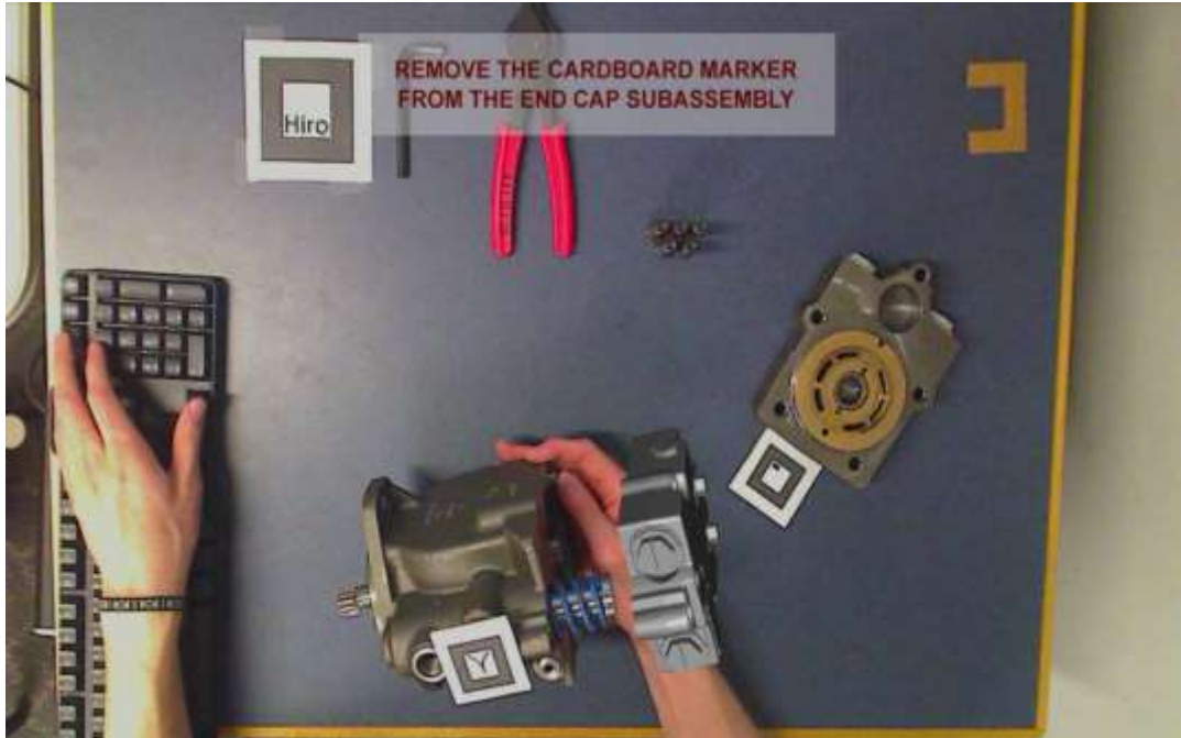
Step 15 – End cap animates up to housing. (Text instructions are not considered an actual assembly step.)
