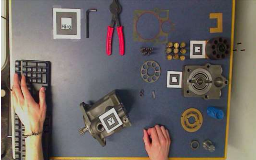
Step 5 – Pins animate into cylinder block.
