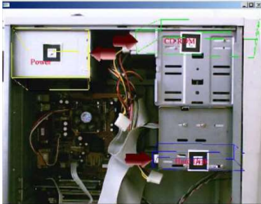
Figure 9. AR assembly utilizing 2D text, 3D arrows, and wireframes [4].
