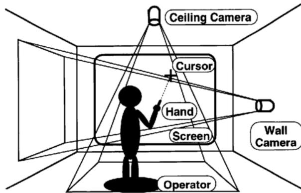
Figure 6: Example ray-casting system system [33]
