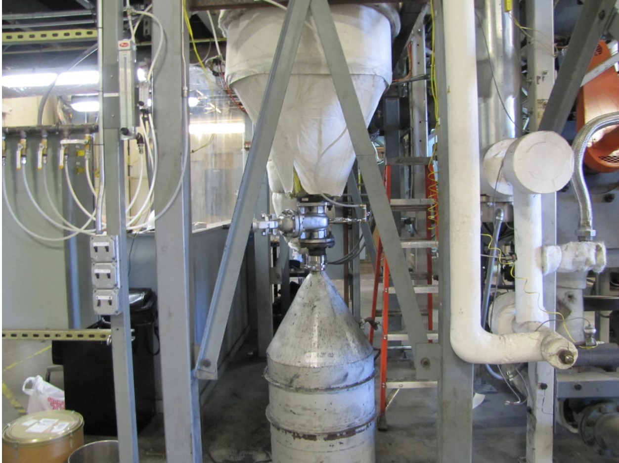
Figure 3.6: Baghouse and chars collection barrel.
