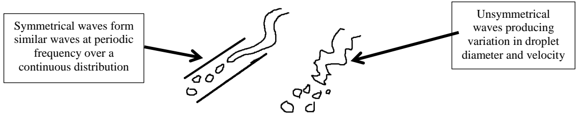
Figure 30: Comparison between global instability producing consistent drops in a narrow range, to local instability creating a range of droplets at various locations
