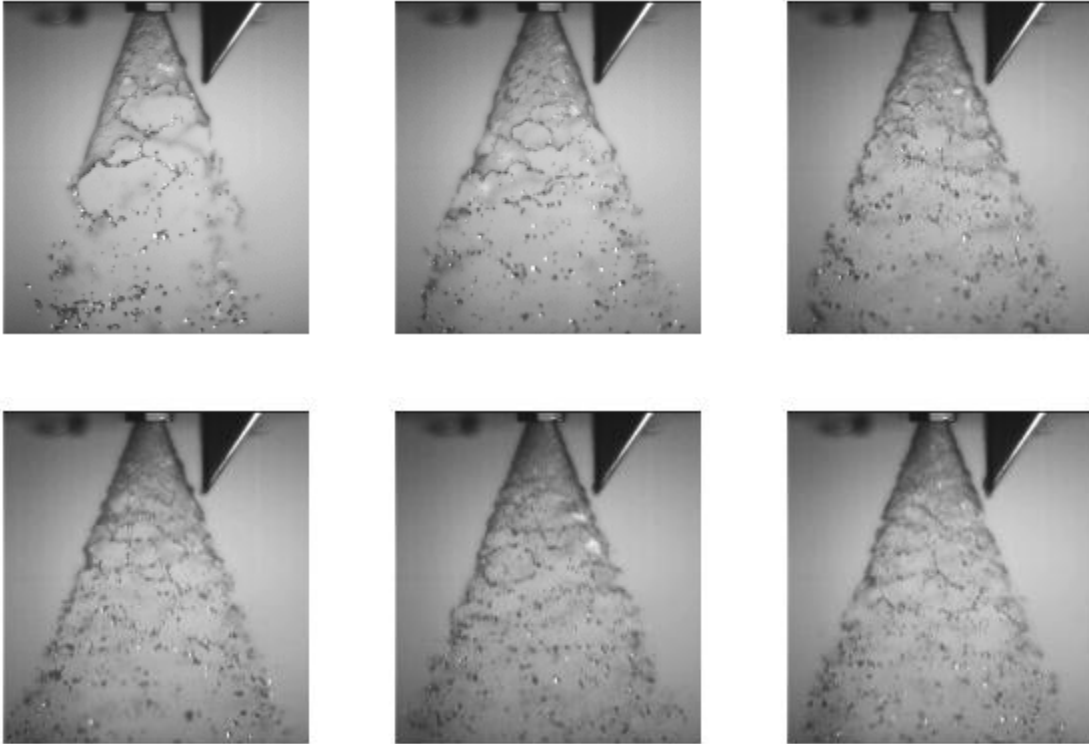
Figure 47: High Speed images of spray breakup for Recessed Length 2 at 12 kHz. Injection pressures are at 68.98, 137.90 and 206.84 kPa (left to right, top panel), and 275.79, 344.74, 413.68 kPa, (left to right, bottom panel) collected at 12 kHz
