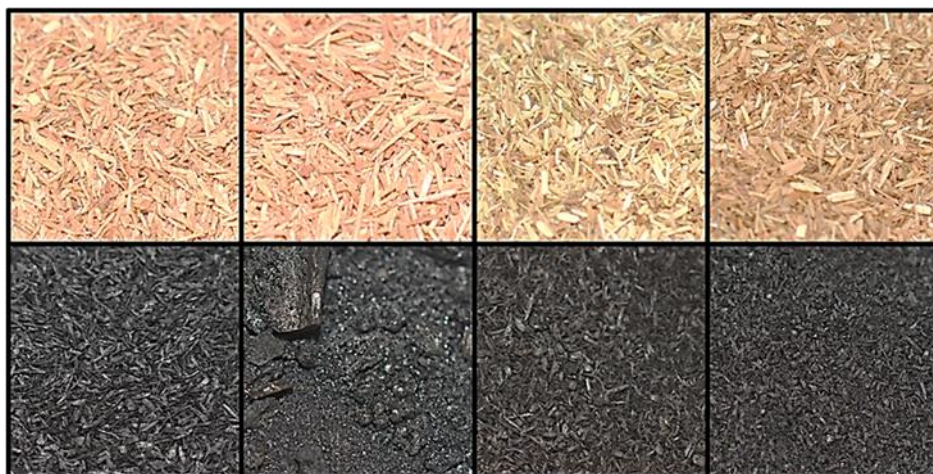
Figure 10: Biomass and biochar comparisons. (Top Row: Red Oak Control, AAEM Passivated Red Oak, Switchgrass Control, AAEM Passivated Switchgrass; Bottom Row: Red Oak Control Char, AAEM Passivated Red Oak Char, Switchgrass Control Char, AAEM Passivated Switchgrass Char)
