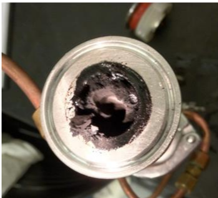
Figure 4: Char formation at high temperature condenser inlet.
