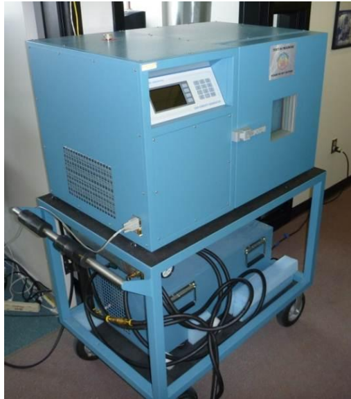
Figure 105. Small environmental chamber actually used for the experiment
