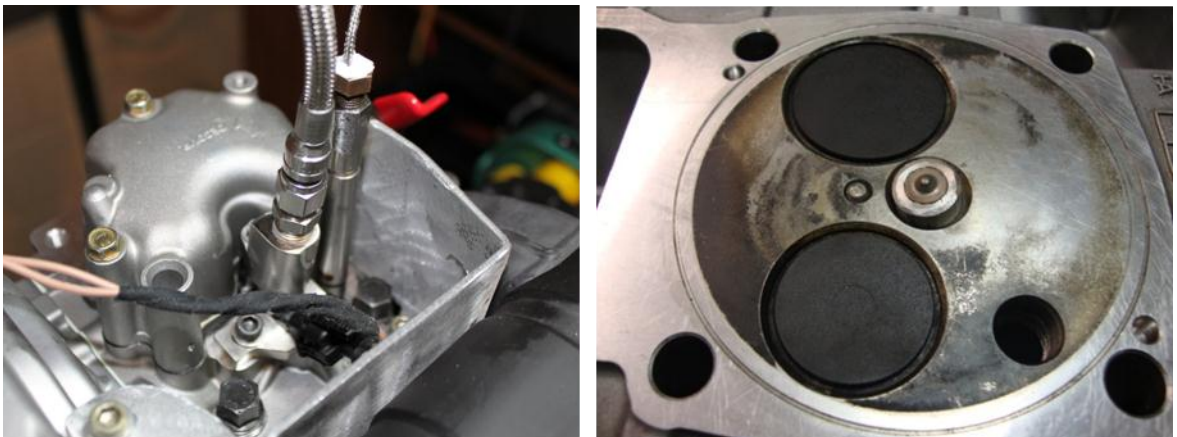
Figure 3.1 – Cylinder head unit with injector, glow plug and pressure transducer
