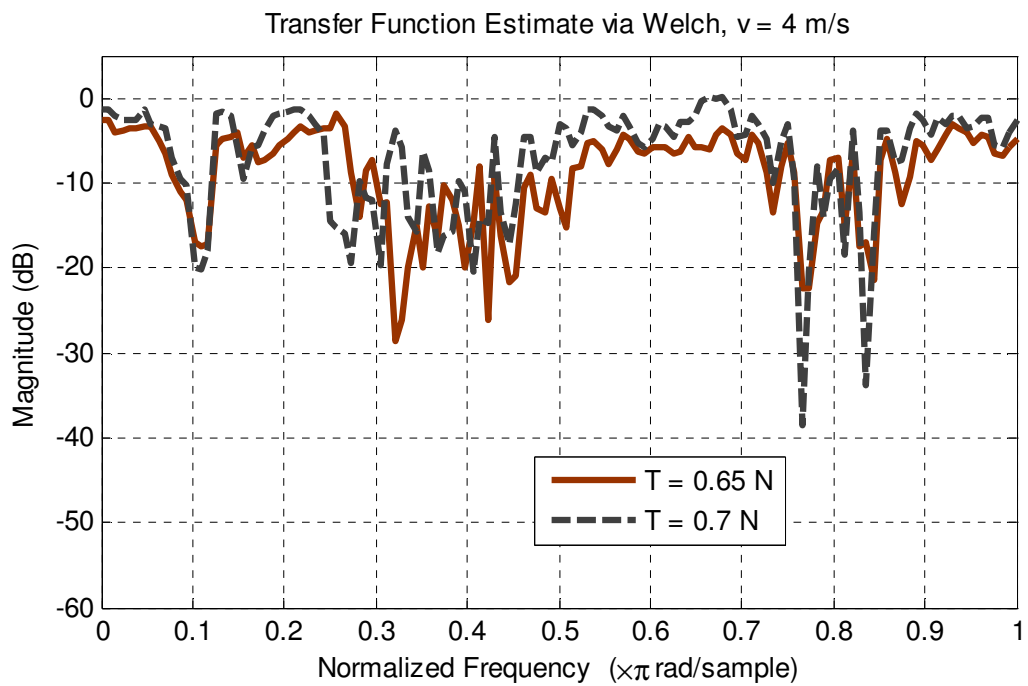
Figure 2.20: Transfer function estimate for T = 0.65 N, 0.7 N & v = 4 m/s
