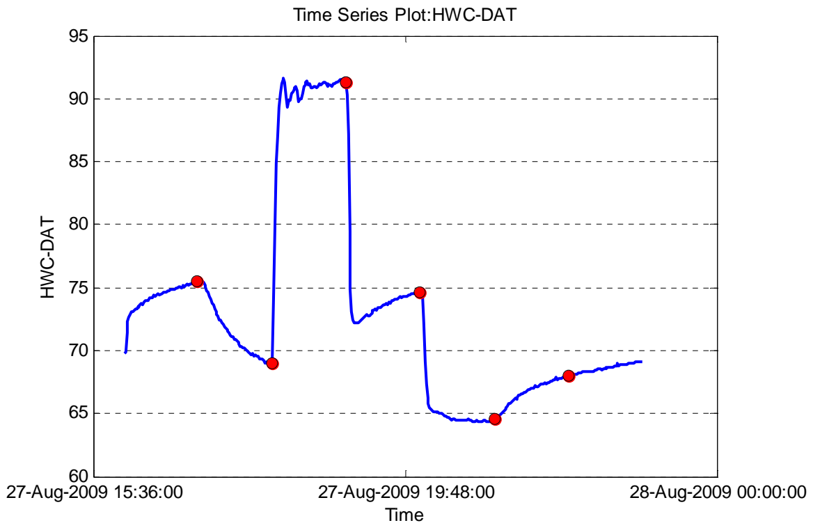
Figure 66. A typical temperature pattern for HWC-DAT
