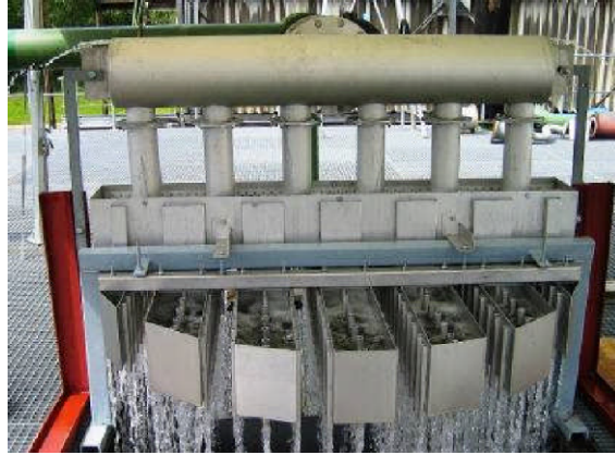
Figure 7.8: Example of liquid distributor (Raschig Jaeger Technologies, 2006).
