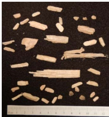
Figure 3.26: Abnormally large red oak chips that were discarded during the manual screening process.
