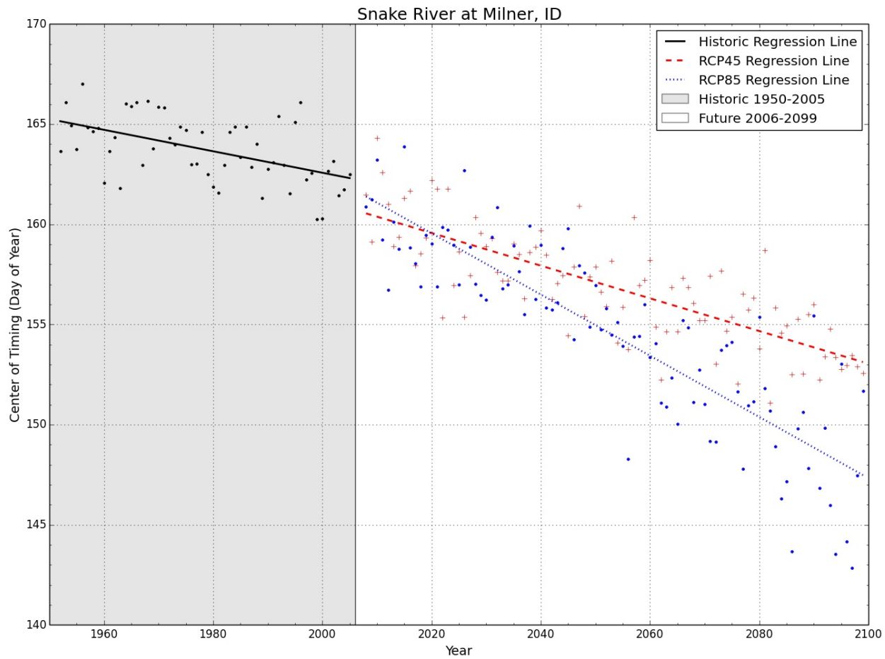
Figure C.9 Center of timing for Snake River at Milner, showing shaded historic (1950-2005) and future (2006-2099)
