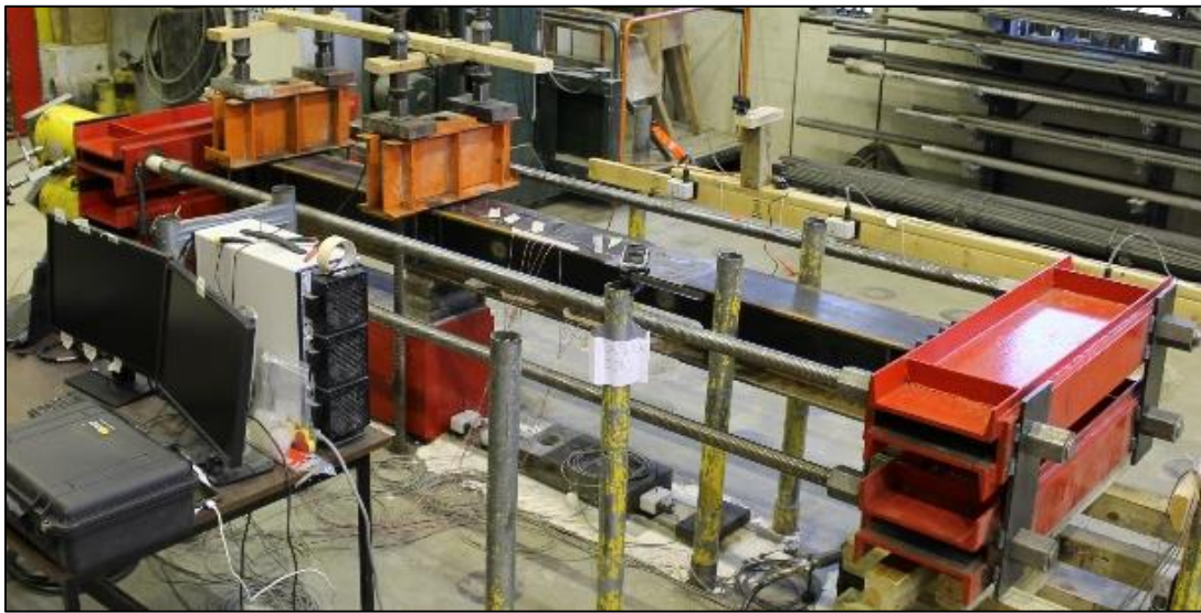
Figure 5.11 Deteriorated abutment test
