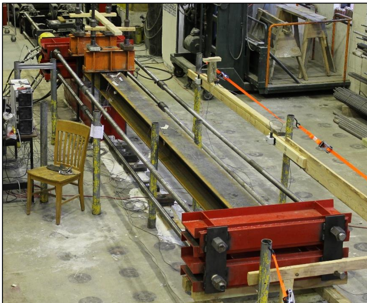
Figure 5.26 Non-deteriorated pile bent test
