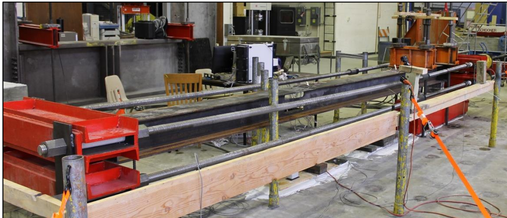
Figure 5.33 Deteriorated pile bent test
