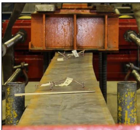
Figure 5.28 Non-deteriorated pile bent LTB failure
