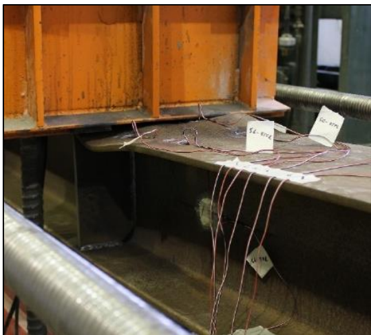
Figure 5.6 Localized failure of base section flange
