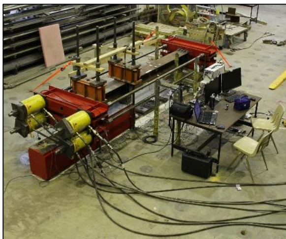
Figure 5.4 Non-deteriorated abutment test
