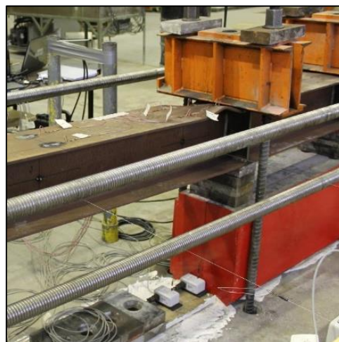
Figure 5.5 Buckling of base section top flange
