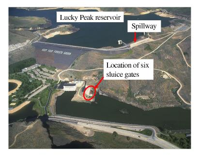
Figure 3.8: Plan view of Lucky Peak reservoir and associated structures.
