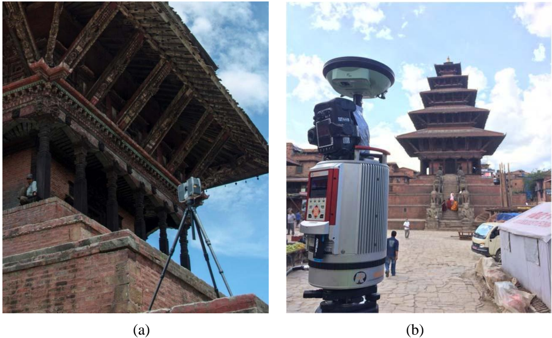
Figure 4.1: Lidar scanning at Nyatapola Temple: (a) Faro Focus 3D X 130 and (b) Riegl VZ-400 laser scanners (Wood et al. 2017a).
