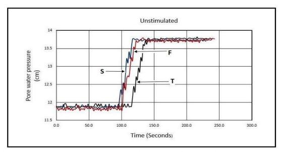
Figure 23. Pore-water pressure head (cm) versus time (sec.) in glass-bead sample during unstimulated impact tests.
