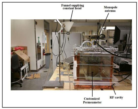
Figure 18. Setup for RF-stimulated hydraulic-conductivity tests
