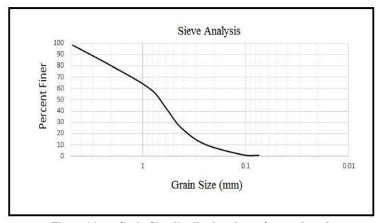
Figure 16. Grain-Size distribution chart of natural sand
