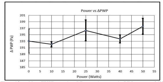
Figure 25. Mean EPWP at various RF-power inputs at the RF frequency of 498 MHz
