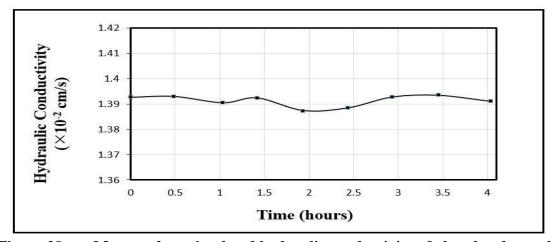
Figure 29. Measured unstimulated hydraulic conductivity of glass-bead sample
