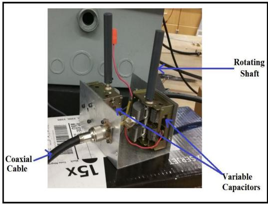
Figure 7. Variable capacitors in the matching network
