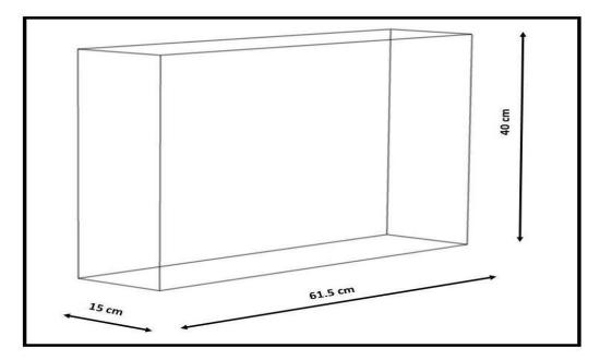
Figure 11. Schematic of the impact-test box with dimension
