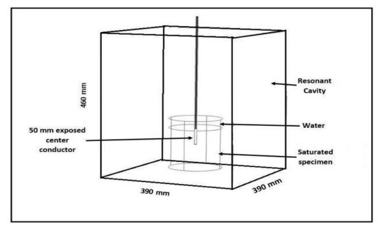
Figure 17. Schematic of the RF-stimulated hydraulic conductivity tests
