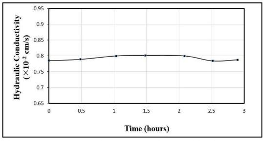
Figure 31. Measured unstimulated hydraulic conductivity of natural-sand sample
