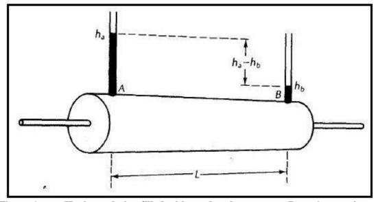
Figure 1. Horizontal pipe filled with sand to demonstrate Darcy's experiment (Fetter, 2001)
