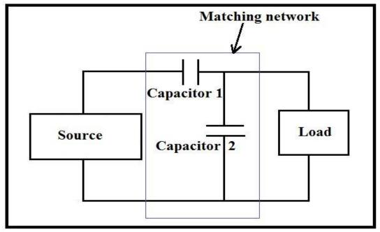
Figure 6. Schematic of impedance-matching network
