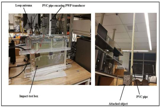
Figure 15. Setup for RF-stimulated impact tests
