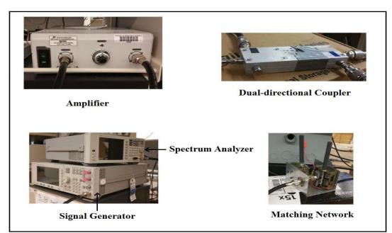
Figure 10. RF-launching setup
