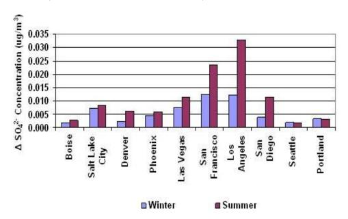
Figure 4.6: Change in a viation  $SO_4^{2-}$  concentration from the base case simulation (RSM999) for the winter and summer.
