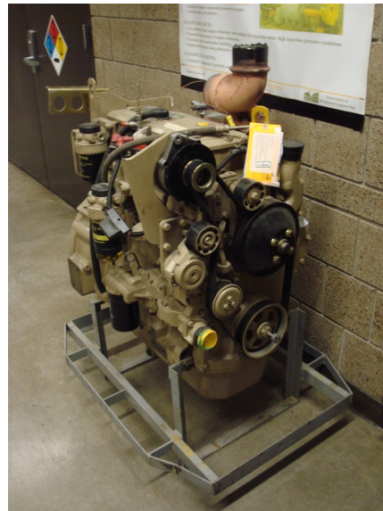
Figure 3.4: Front-right view of another John Deere 4045HF475 diesel engine
