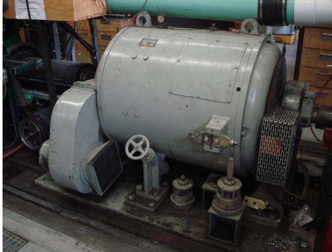
Figure 3.5: General Electric 112 kW dynamometer
