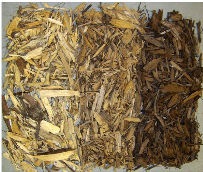
Figure 11: Loblolly pine slash biomass torrefied at 180°C, 215°C, and 250°C (left to right).
