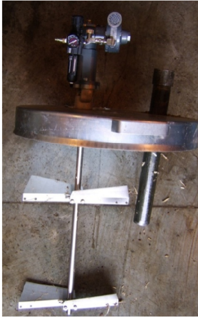
Figure 6: Modified pneumatic mixers used for water washing.
