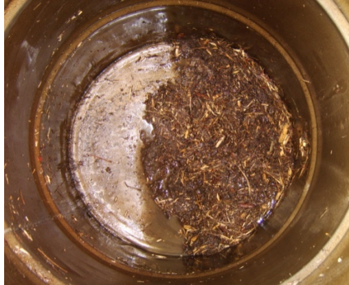
Figure 8: Sand (left) and saturated biomass (right) collected at the bottom of a drum.
