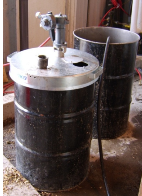
Figure 7: Drums used for washing. The drum on the left has the mixer inserted.
