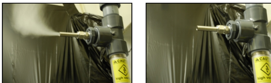
Figure 18: ESP operation. Left: OFF aerosol bio-oil escaping. Right: ON, complete aerosol removal.
