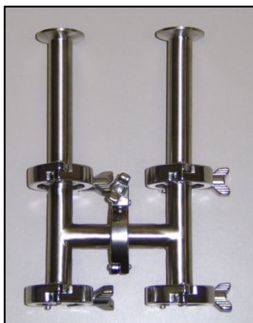
Figure 17: Stainless steel condenser in “H” shape.
