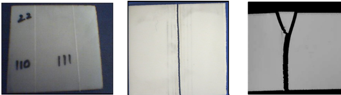
Fig 3.5 (a): Photographs of scribing (left), (b): controlled (center) and (c): uncontrolled fracture (right).
