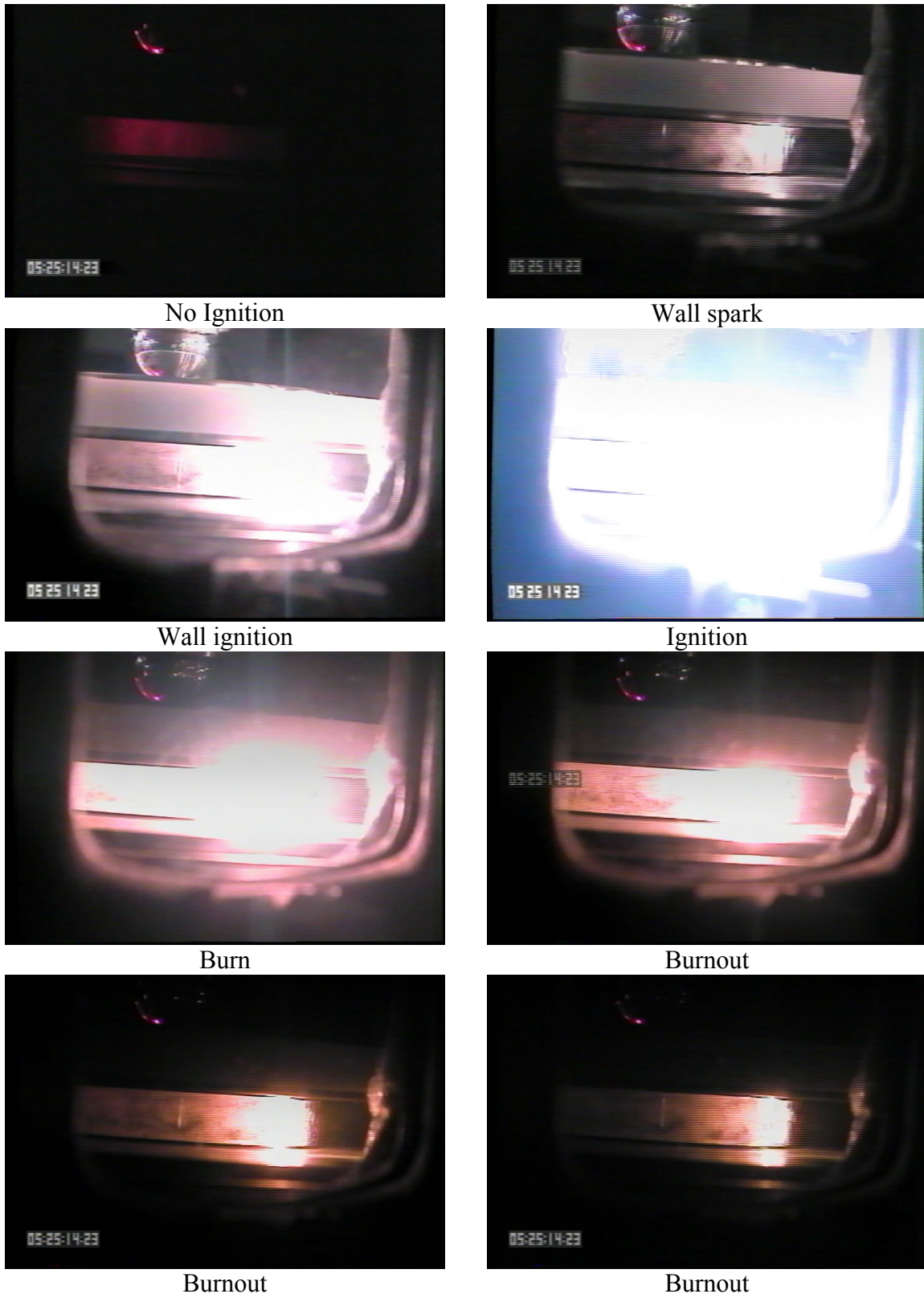
Figure 6.7. Ignition development in drop tower for Al ( d_{32}=31.87 \mu\text{m} ).
