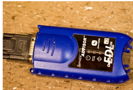
Figure 3.2 - USB CAN2 250 adapter used to connect to L14 ECU/EDU.
