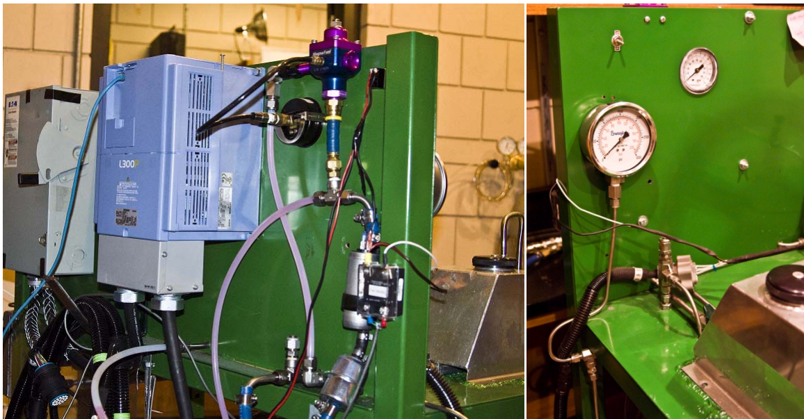
Figure 3.5 - Fuel supply pump and fuel filter (left), hand valve and dial gauges (right).
