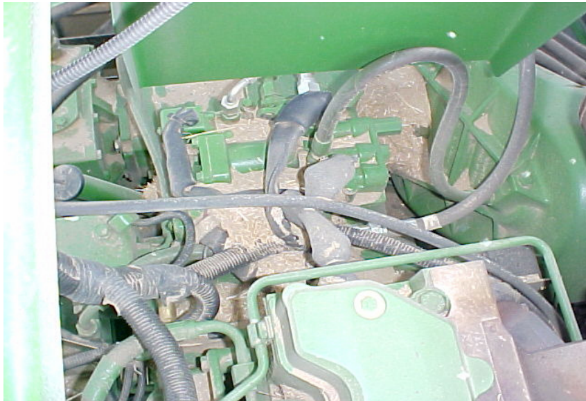
Figure 5. Harvester engine compartment with debris accumulation
