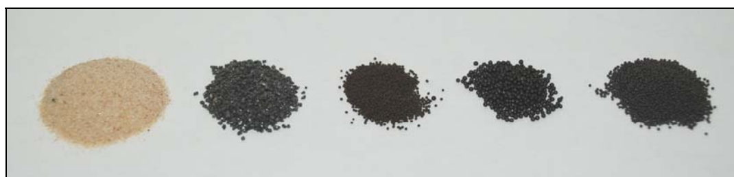
Figure 38. Sand, silicon carbide, alumina ceramic and steel shot heat carrier examples
