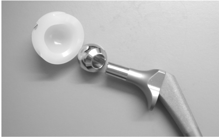
Figure 1- 1. Major components of total hip joint replacement; polymeric acetabular, femoral head, and femoral stem
