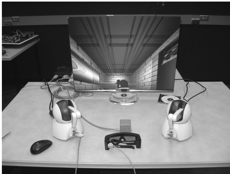
Figure 3.2. Hardware setup for immersive virtual reality system
