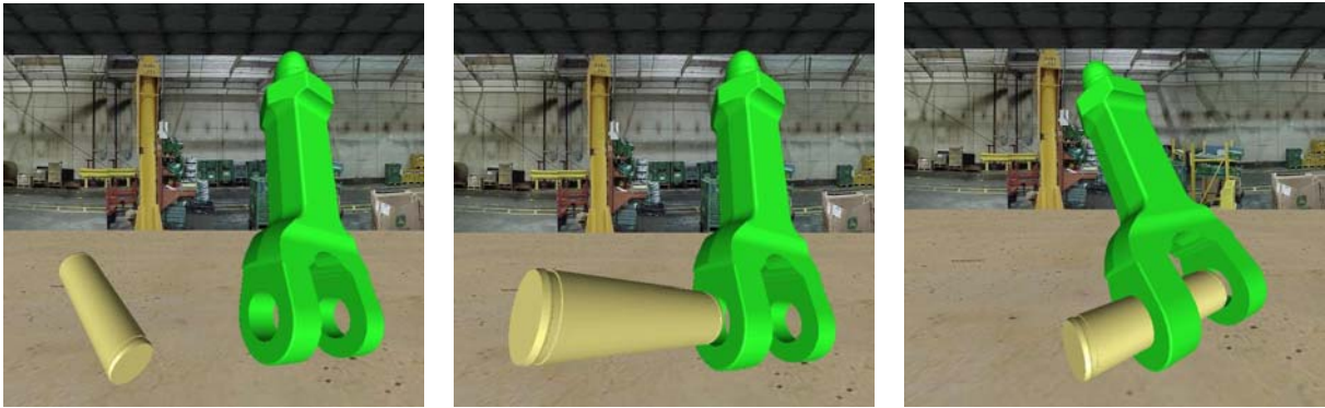
Figure 5: Assembling Pin and Center-link using SHARP
