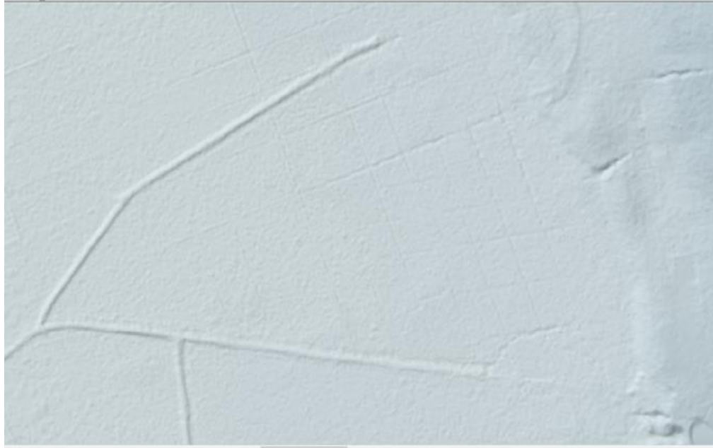
Figure 3.4. Digital Elevation Model Layer for Project Area One. The above image shows the DEM layer and the hillshade layer created from the LIDAR ground points for the study area. The grid lines often forming rectangles are located in the middle with lines extending to the north and east.
