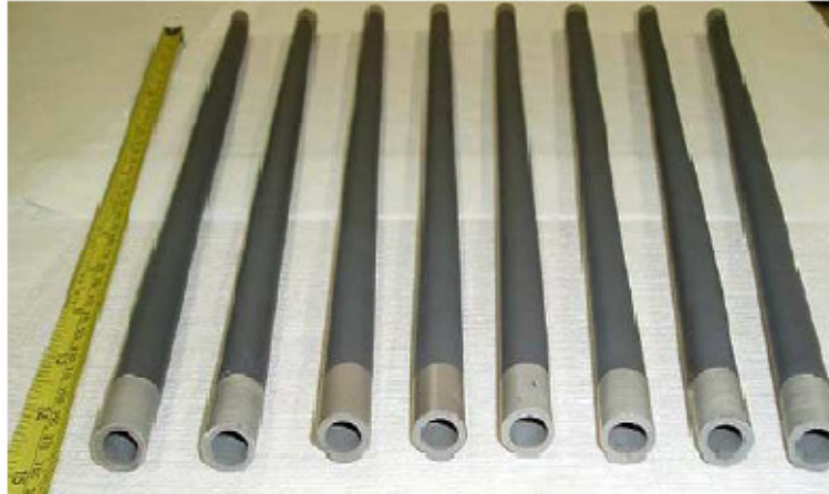
Figure 16. Tubular cells fabricated, in part, by extrusion. The electrolyte was extruded, then the anode was dip coated on the inside of the tube, the assembly was fired, the cathode was slurry painted on, and the total assembly was fired again [48].
