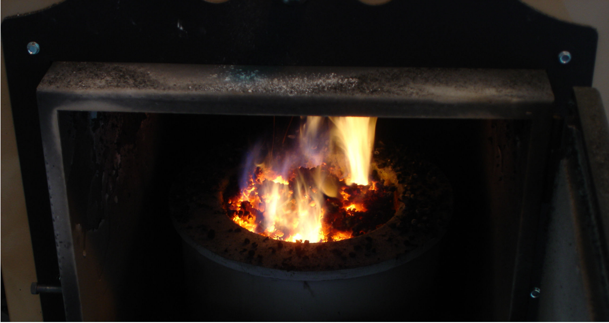
Figure 10: LDJ 620-10 in operation - notice glowing clinkers surrounded by flames
