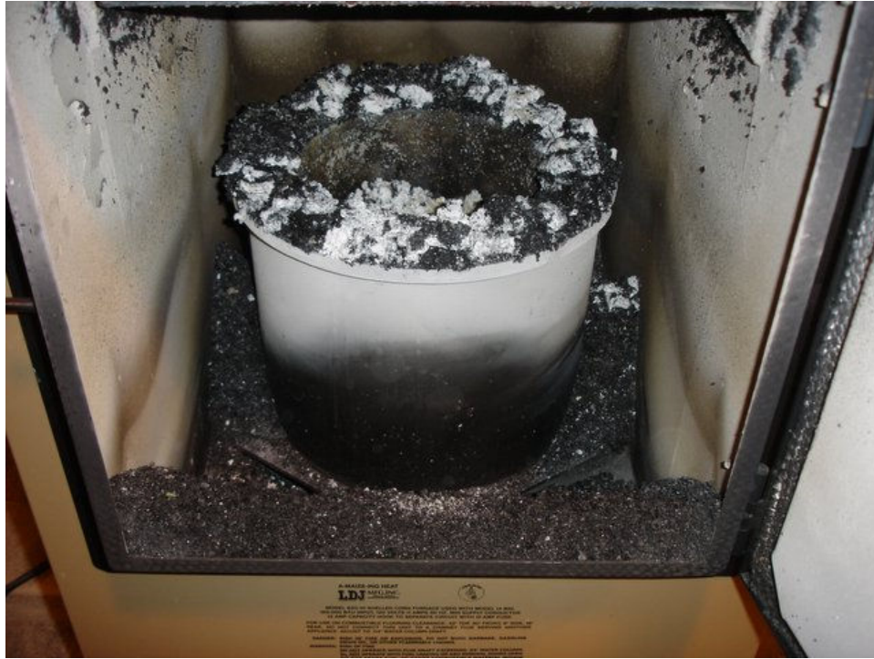
Figure 2: An abundance of clinker from using a corn furnace
