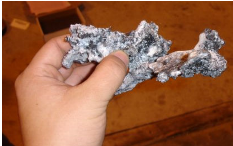
Figure 1: A large clinker formed by burning corn
