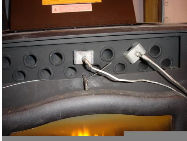
Figure 6: Country Flame Harvester heat exchanger with thermocouples visible
