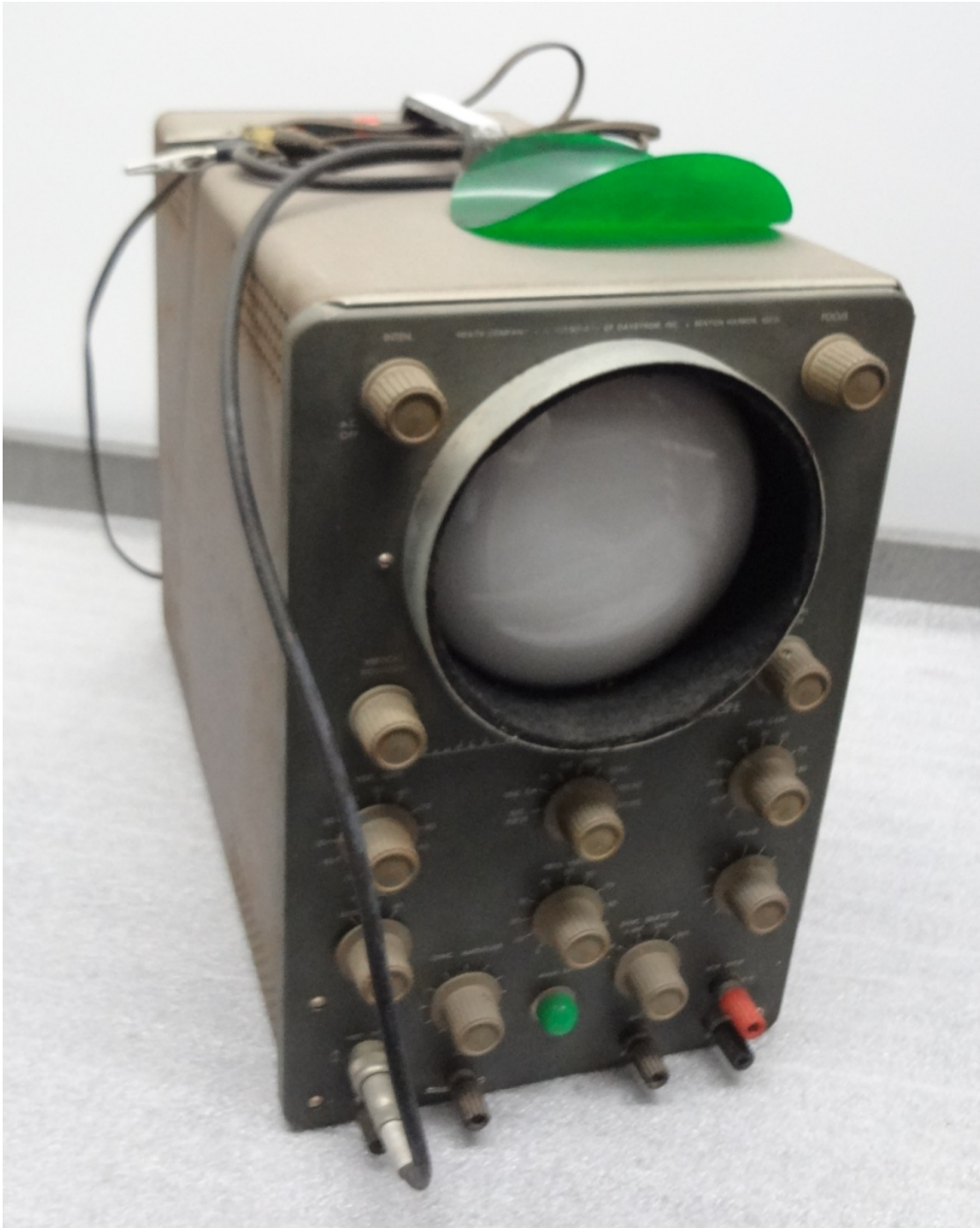
Figure 5.2 Heathkit Laboratory Oscilloscope, ca. 1960. Heathkit served as one of the most popular home electronics kit manufacturers in the country, offering affordable, well-crafted equipment to amateur tinkerers. Photo by author. Courtesy of The Strong®, Rochester, New York.
