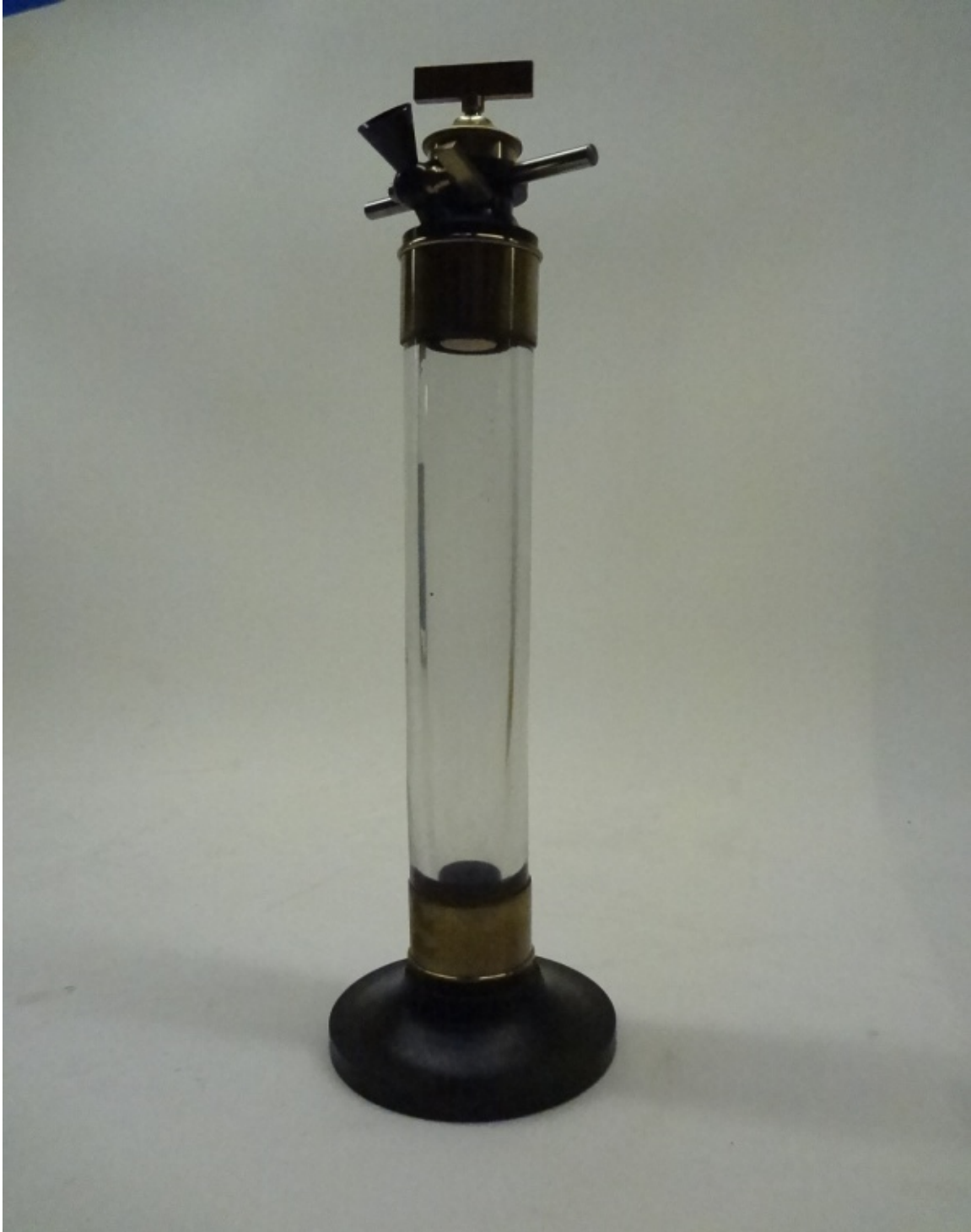
Figure P1.2: European Cartesian Apparatus from the nineteenth century. Featuring an ornate brass base large enough for performing demonstrations in lecture halls, this apparatus was great for lectures but less practical for everyday classroom use. Photo by author. Courtesy Smithsonian Institution National Museum of American History Physical Sciences Collection.
