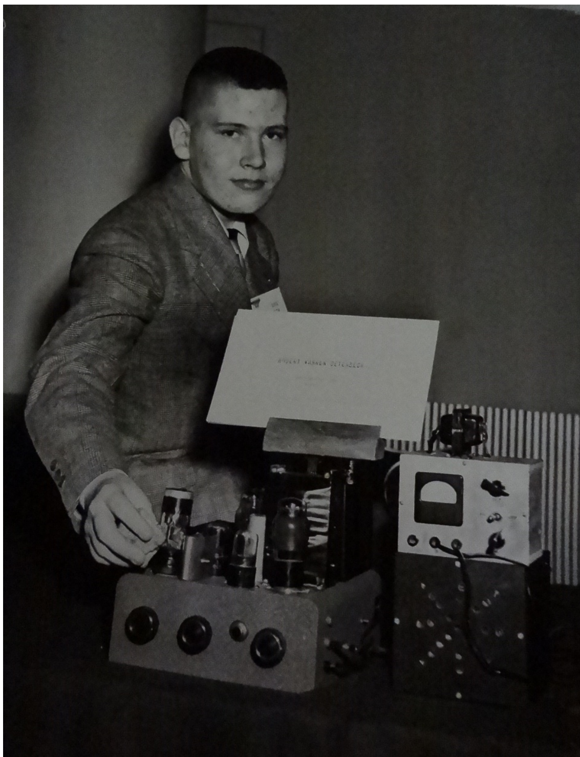
Figure 5.17 1950 Science Talent Search finalist Robert Warren Detenbeck with his exhibit, "Scintillation Counter Converts Tiny Flashes of Light Produced by Radioactive Emanations on a Fluorescent Screen into Electrical Impulses." Courtesy Society for Science and the Public Photograph Collection.
