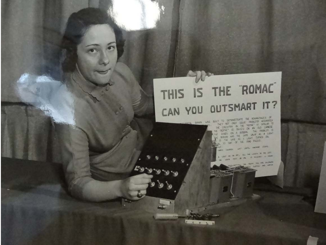
Figure 4.9 Rosemary Och with her mechanically actuated computer, “ROMAC.” Courtesy Society for Science and the Public Photograph Collection.
