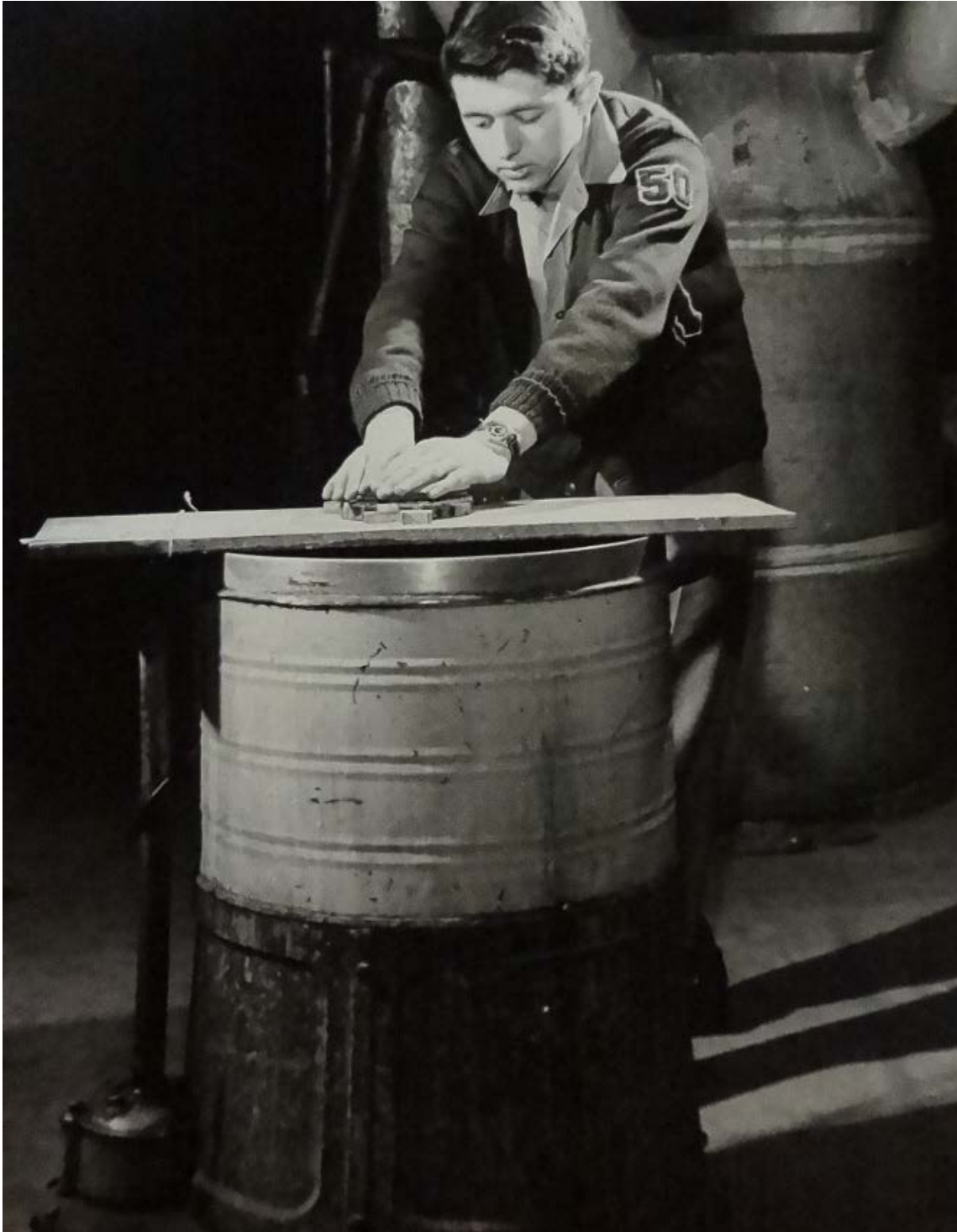
Figure 4.17 Joel Dean Finegan grinding his telescope mirror on his mother's washing machine. According to the photo description, "The family wash waited while he ground." Courtesy Society for Science and the Public Photograph Collection.
