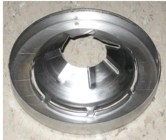
Figure 3.6 Standard F3 air swirler used in the Beckett AF burner.
