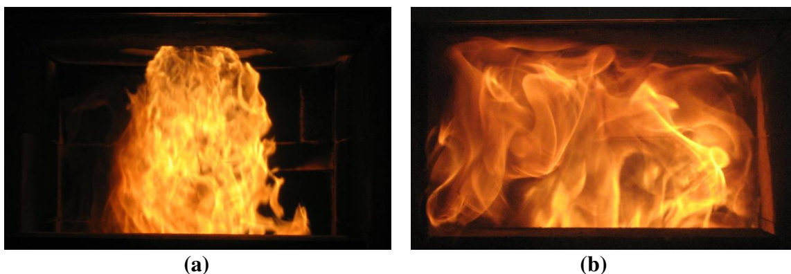
Figure 3.4 Photographs of a (a) stabilized fuel oil flame and (b) unstabilized pyrolysis oil flame in a Beckett AF burner with minor modifications.
