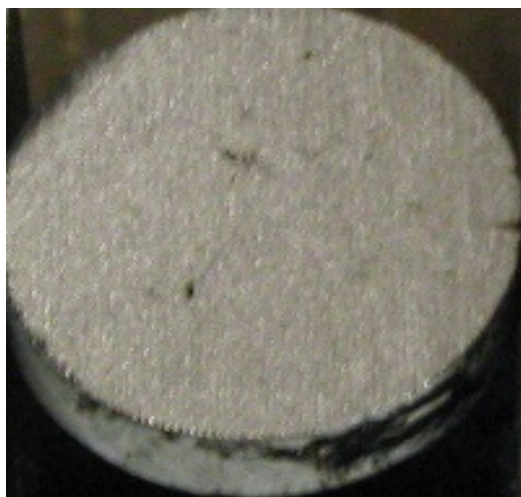
Figure 9: Digital photograph of optimally laser-sintered coupon
