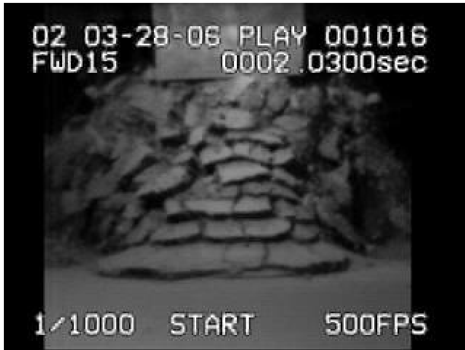
Figure 4.5: Soil bin test – 178 mm sweep, 2.68 m/s, 76 mm depth, high moisture (8.3% d.b.), high compaction (1,100 kPa)
