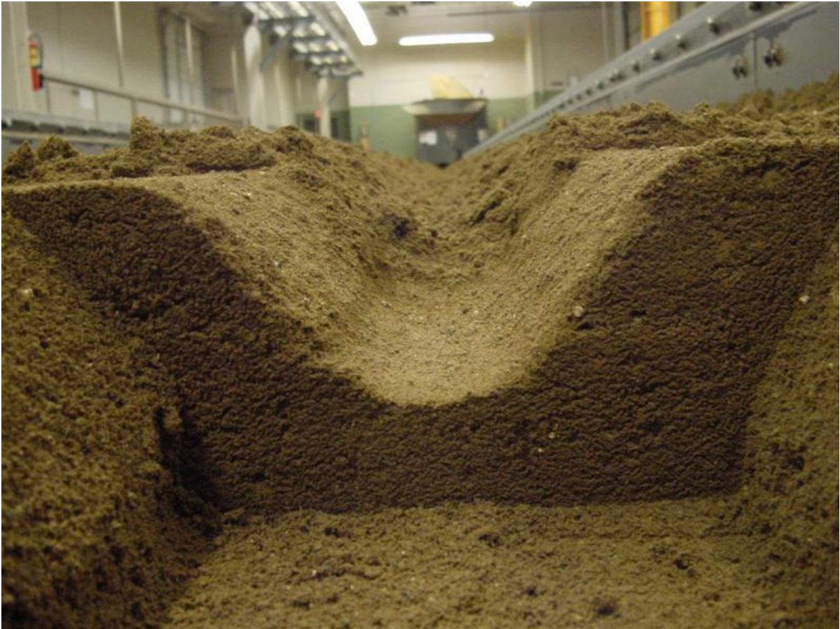
Figure 3.2: Flat bar example trench profile with loose soil cleared away
