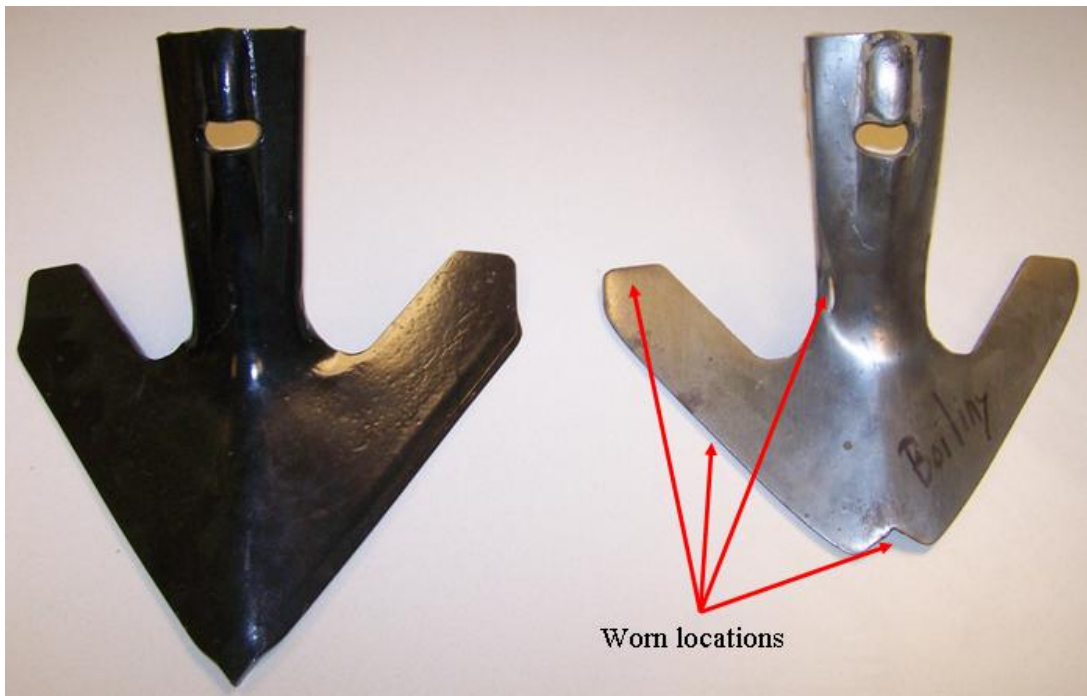
Figure 7.15: Field cultivator standard – example of new and worn 254mm sweep
