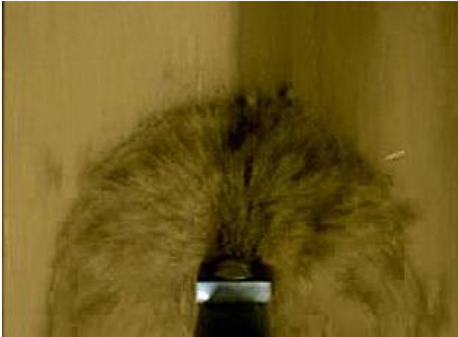
Figure 3.3: Image of soil failure, 51 mm depth, 2.68 m/s, low compaction (200 kPa)
