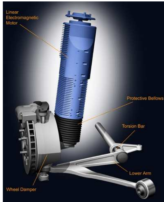
Figure 1.2 The Bose fully-active suspension system
