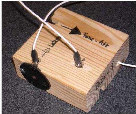
Figure 2.6 Floor region accelerometer module showing a 3-axis set
