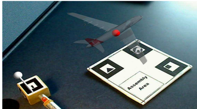
Figure 19: When the CG button is activated, the models become transparent and the center of gravity is represented by a small red sphere.
