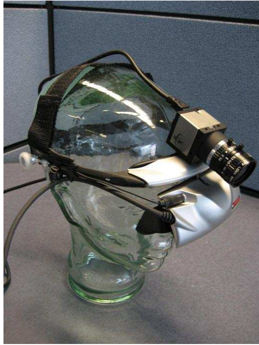
Figure 7: One example of a video see-through display using an HMD and a camera.
